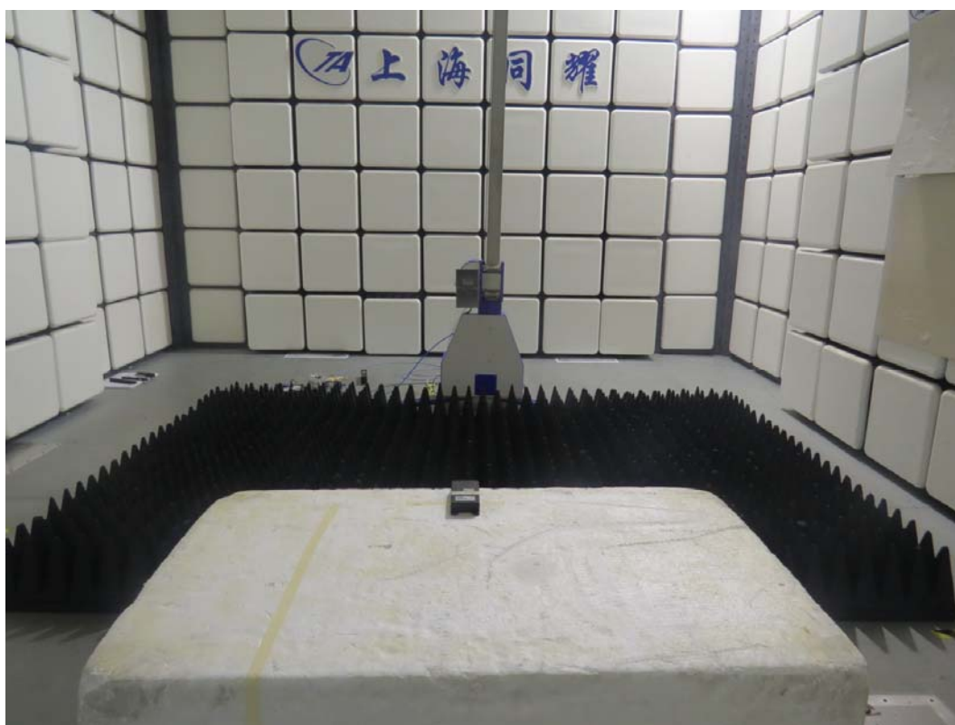
Picture 1 Radiated Emission Test Setup
