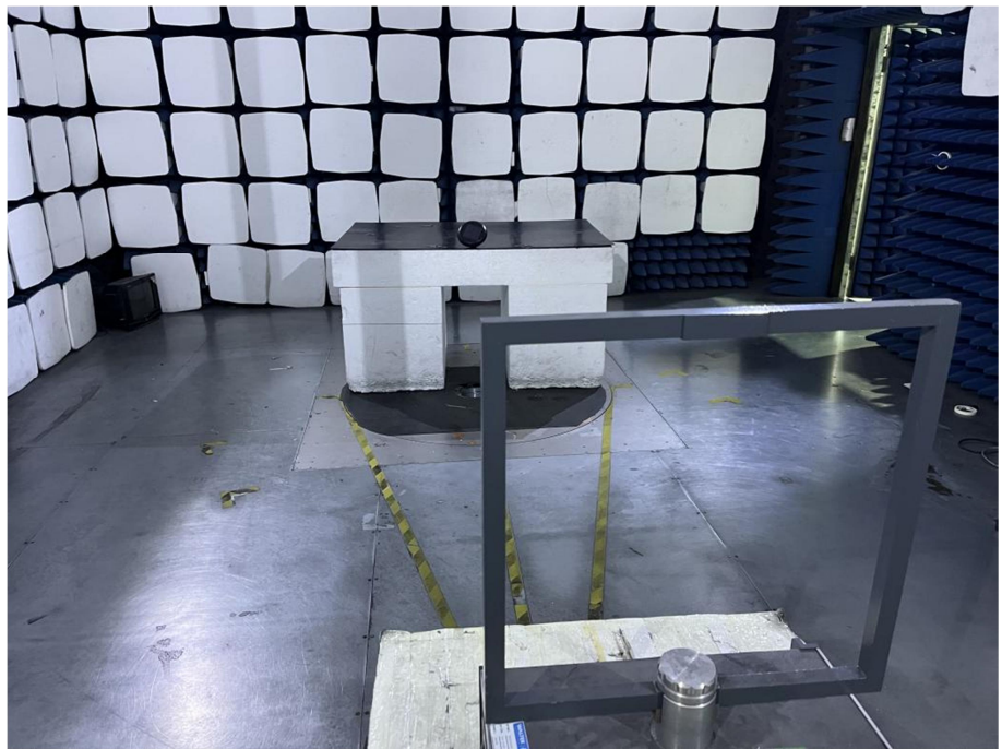
Radiation Emission Test Setup (Below 30MHz)
