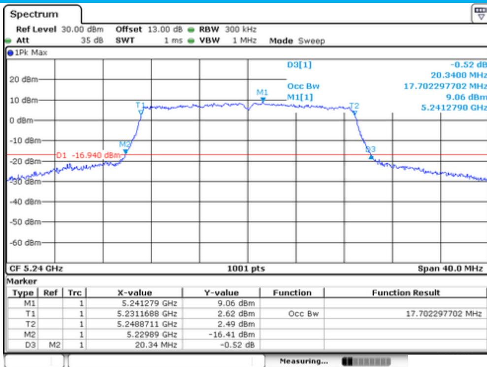
Emission Bandwidth&amp;99% Occupied Bandwidth UNII Band III
