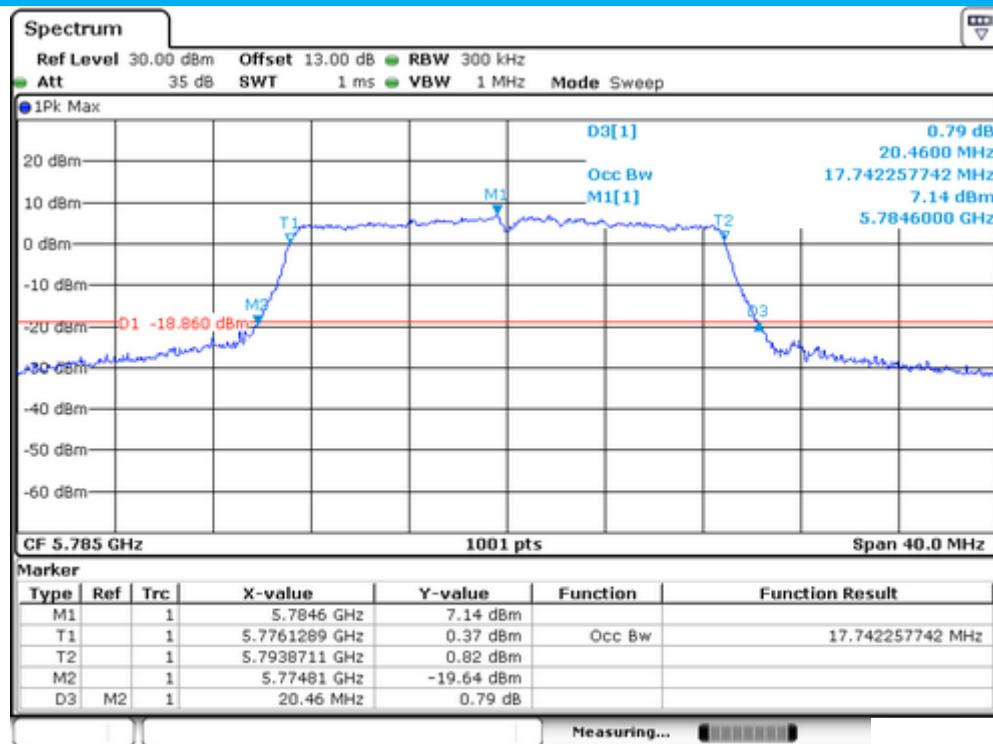
Emission Bandwidth&amp;99% Occupied Bandwidth UNII Band III
