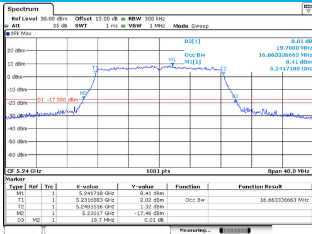
Emission Bandwidth&amp;99% Occupied Bandwidth UNII Band III
