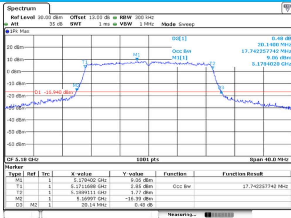
Emission Bandwidth&amp;99% Occupied Bandwidth UNII Band I
