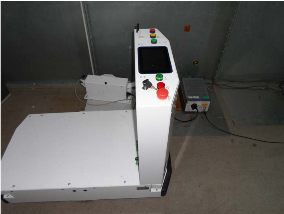
Measurement of Conducted Emission Test Set Up
