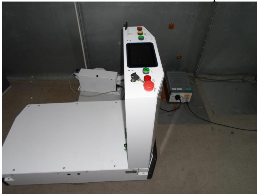
Measurement of Conducted Emission Test Set Up
