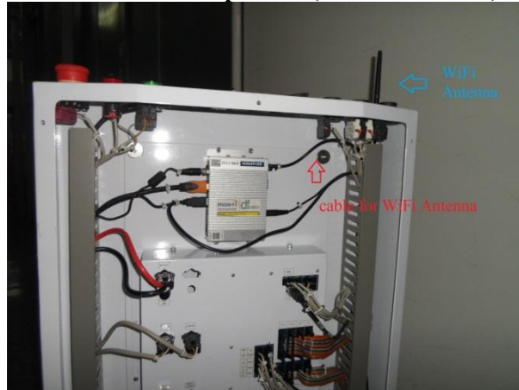
Inside View of the product (Antenna location)
