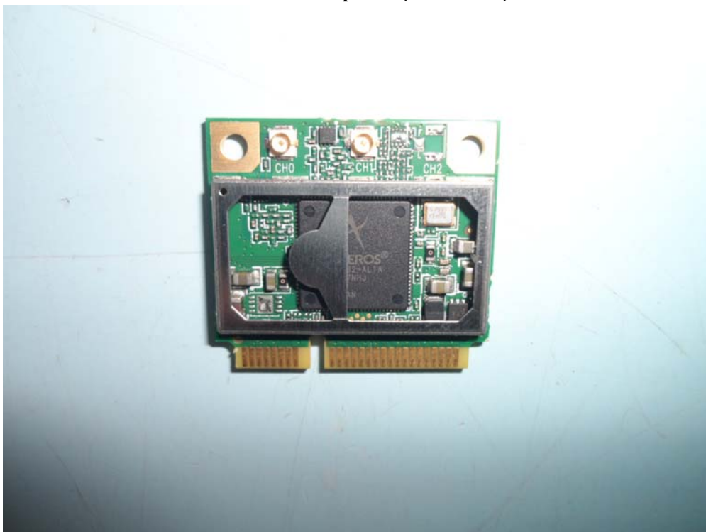
Inner Circuit Top View(RF Module)
