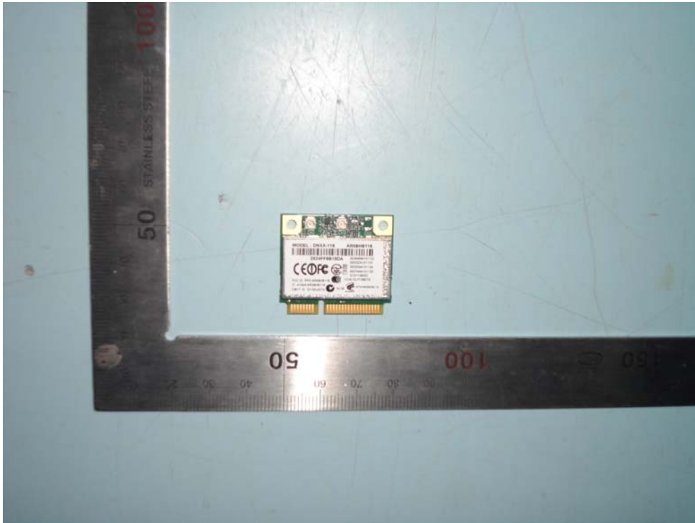
Inner Circuit Top View(RF Module)
