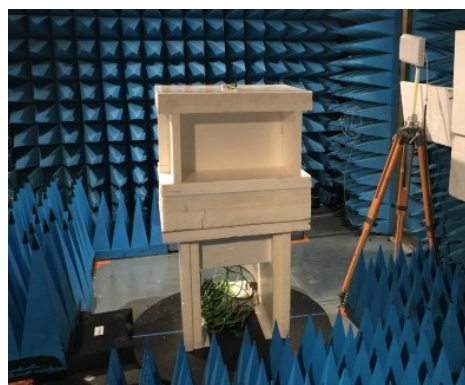
General Test setup in anechoic chamber >1GHz
