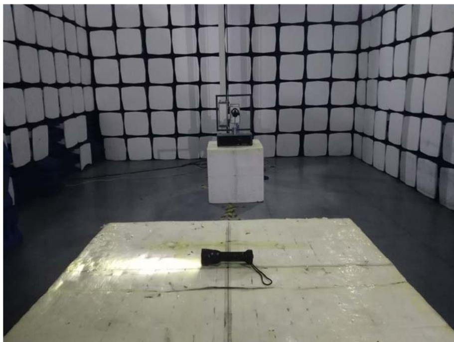
**Radiation Emission Test Setup (30MHz to 1GHz)**
