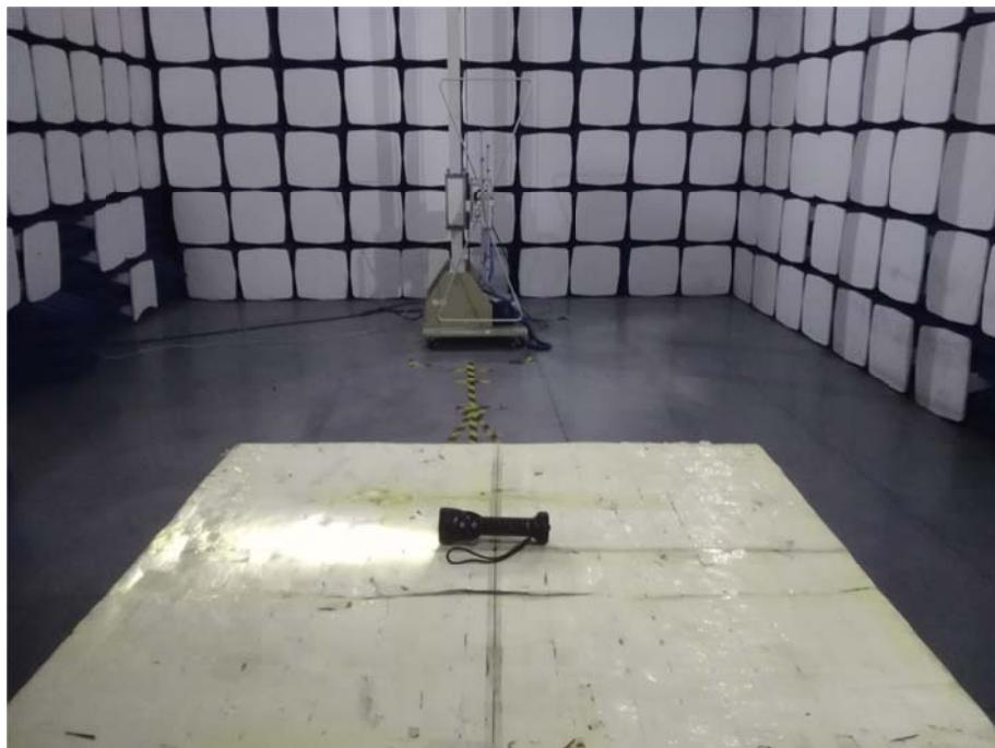
**Radiation Emission Test Setup (1GHz to 18GHz)**
