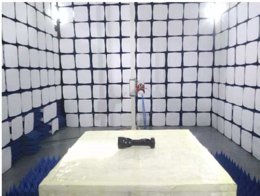
**Radiation Emission Test Setup (Above 18GHz)**
