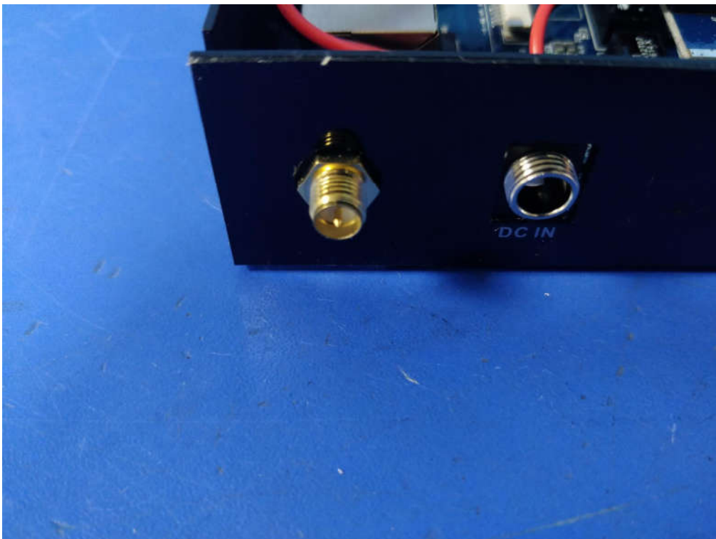
Close view for SMA antenna connector
