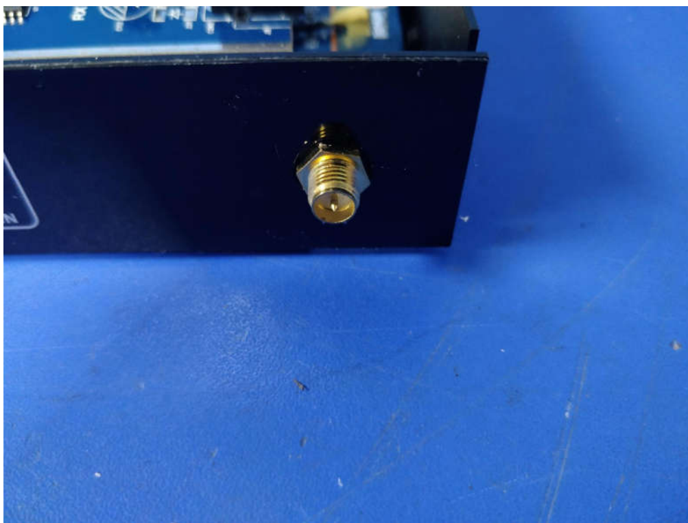
Close view for SMA antenna connector
