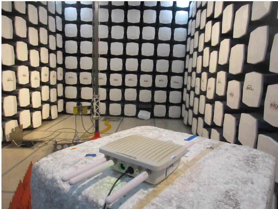
**1.5 Radiated Spurious Emission above 18-26.5 GHz Front View**
