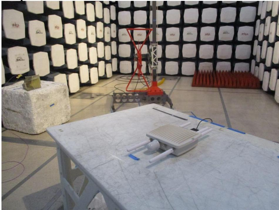
**1.3 Radiated Spurious Emission above 1-18 GHz Front View**
