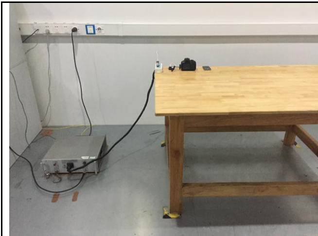
Conducted Emissions Test Setup Front View
