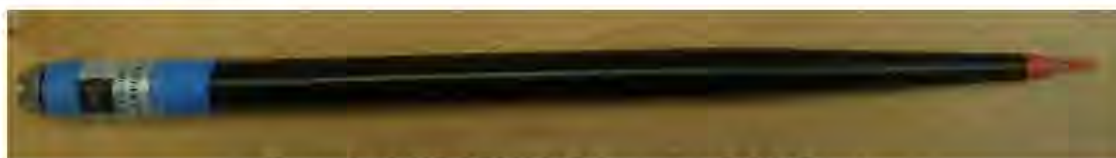
Figure 1 – MVG COMOSAR Dosimetric E field Dipole
