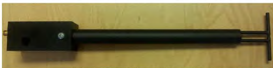
Figure 1 – MVG COMOSAR Validation Dipole
