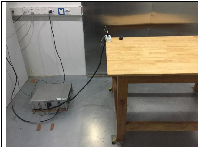
Conducted Emissions Test Setup – Front View
