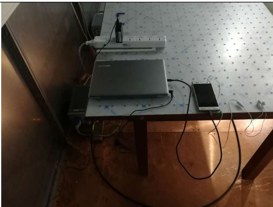
Conducted Emissions Test Setup (with charger)
