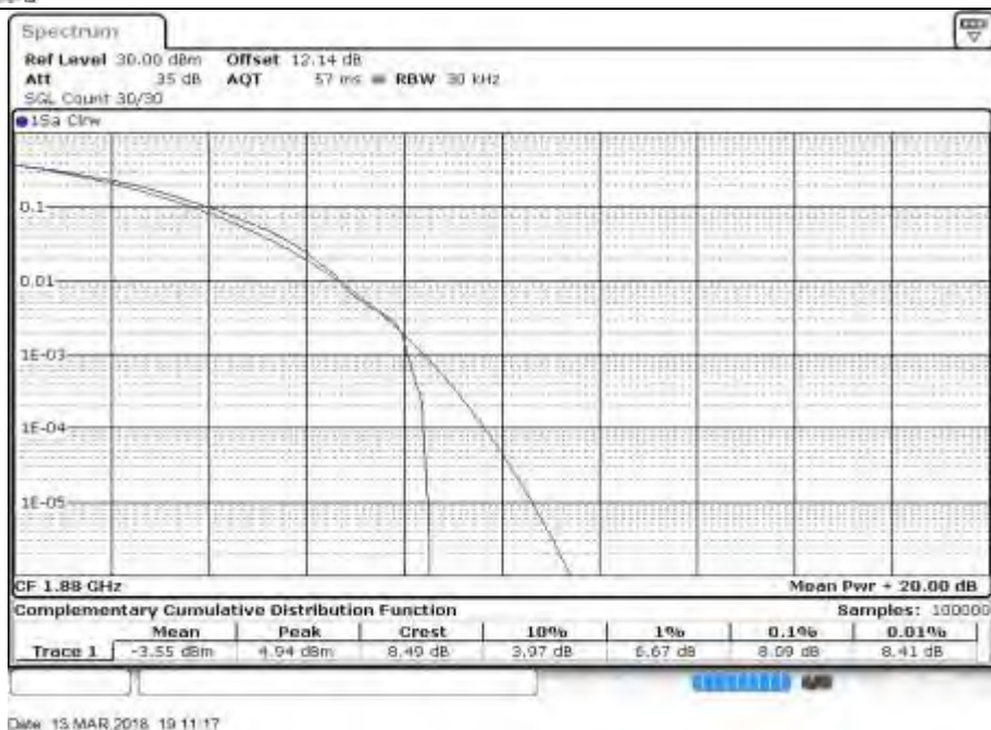
Peak-Average Ratio Plot(20MHz BW,QPSK,Band 2-mid Channel)
