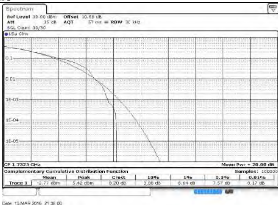
Peak-Average Ratio Plot(15MHz BW,QPSK,Band 4-mid Channel)
