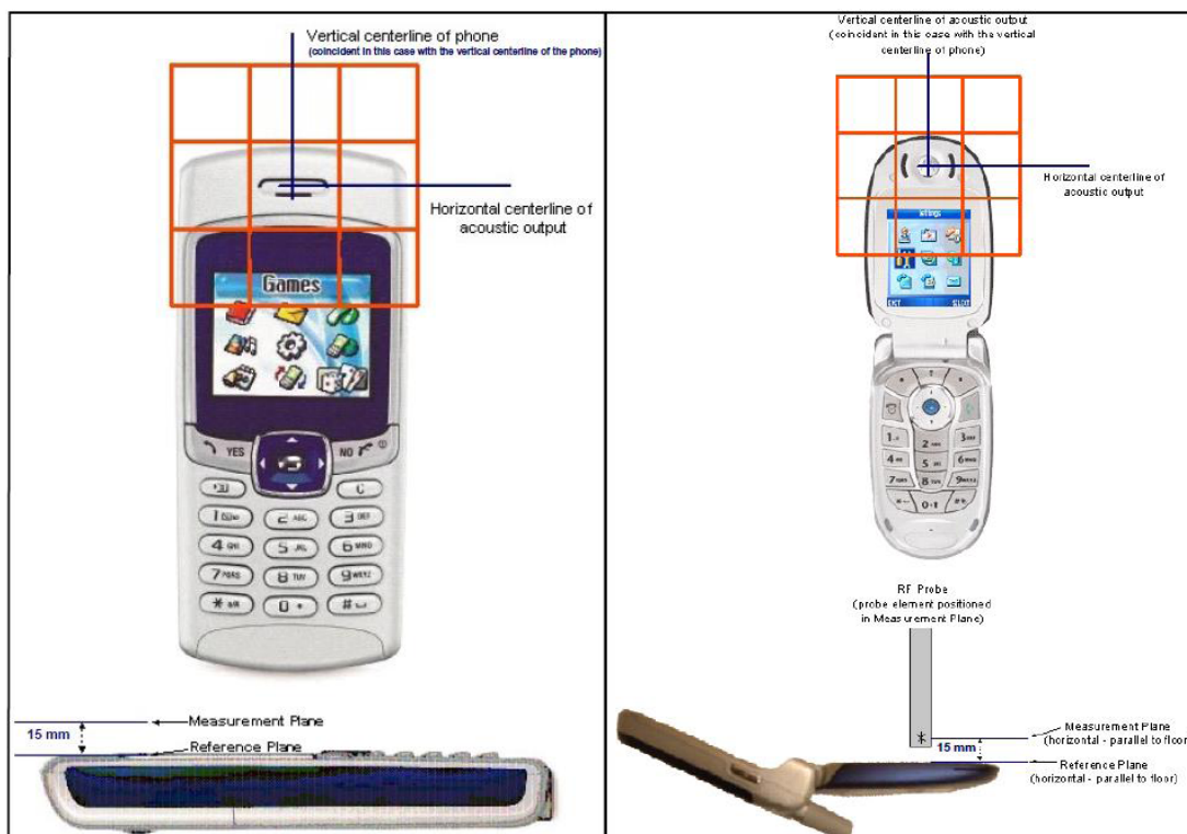
WD reference and plane for RF emission measurements
