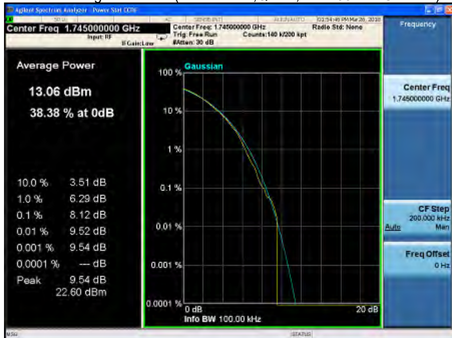
Peak-Average Ratio Plot(1.4MHz BW,16QAM,Band 66-mid Channel)
