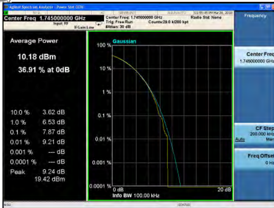
Peak-Average Ratio Plot(3MHz BW,QPSK,Band 66-mid Channel)
