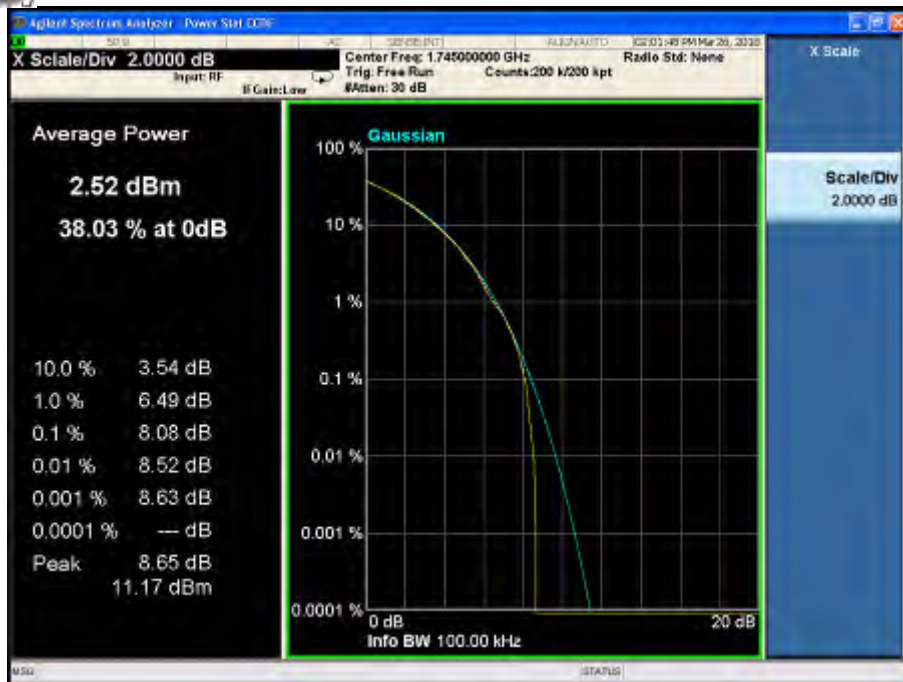
Peak-Average Ratio Plot(20MHz BW,QPSK,Band 66-mid Channel)
