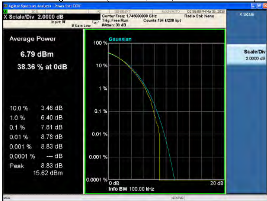
Peak-Average Ratio Plot(5MHz BW,16QAM,Band 66-mid Channel)
