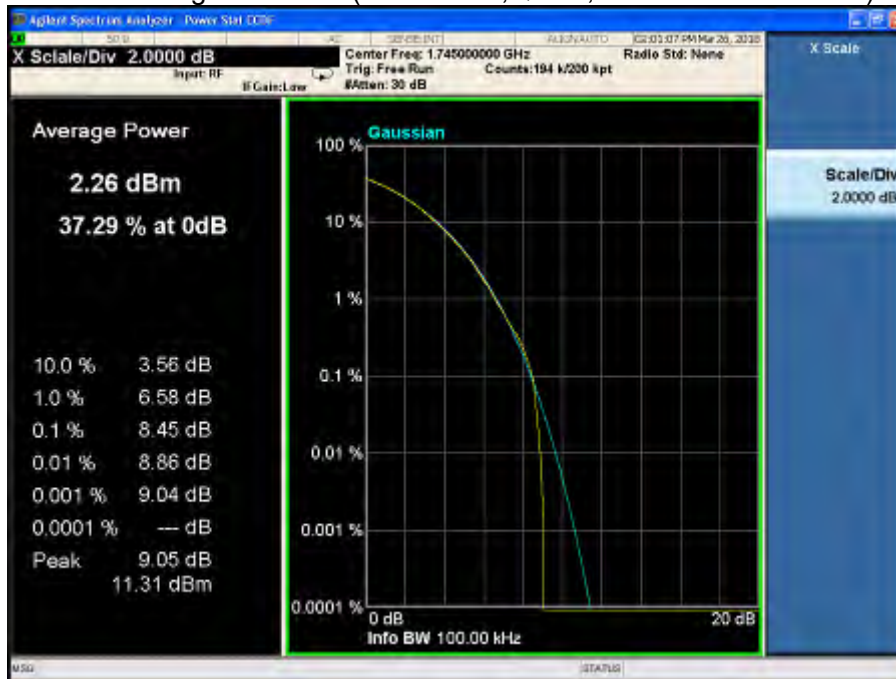
Peak-Average Ratio Plot(15MHz BW,16QAM,Band 66-mid Channel)
