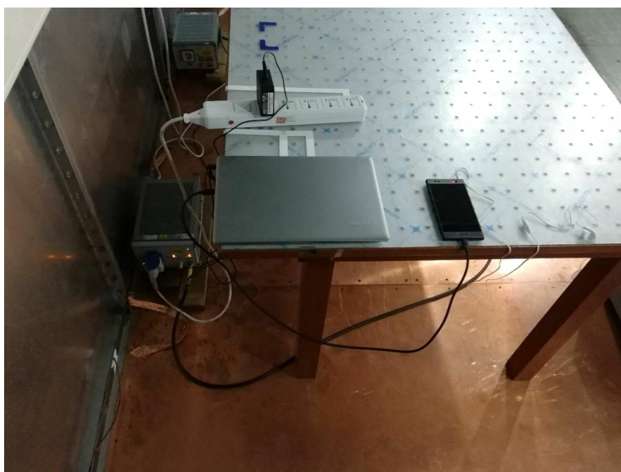
Conducted Emissions Test Setup (with charger)
