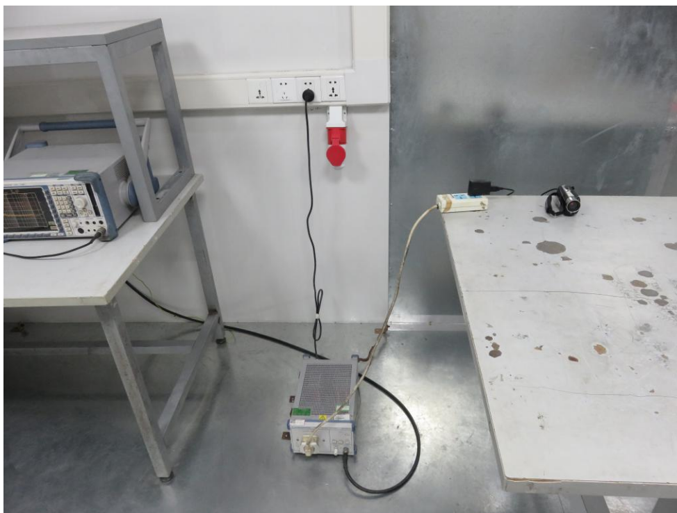
Photo of Radiation Emission Test
