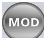
6、Mode switch , When the USB is inserted, the switches are switched in turn → AUX BT USB
