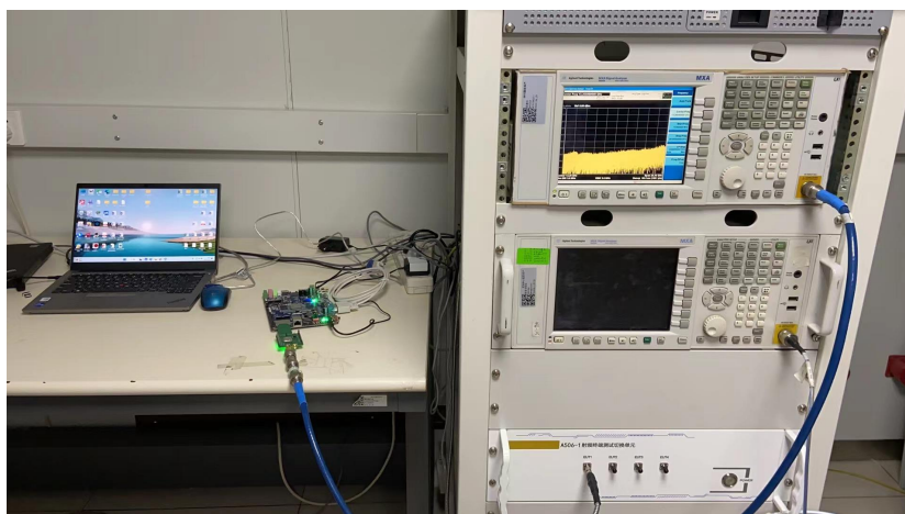
RF Conducted Test setup (BT/WIFI)
