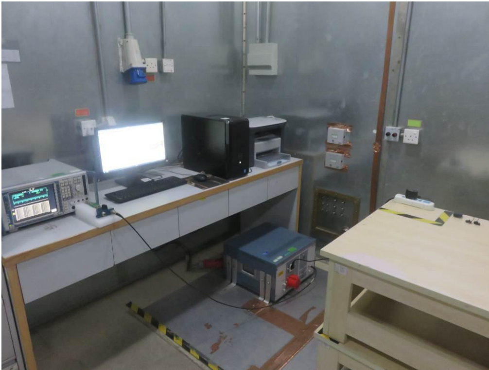
FCC RADIATED EMISSION TEST SETUP
