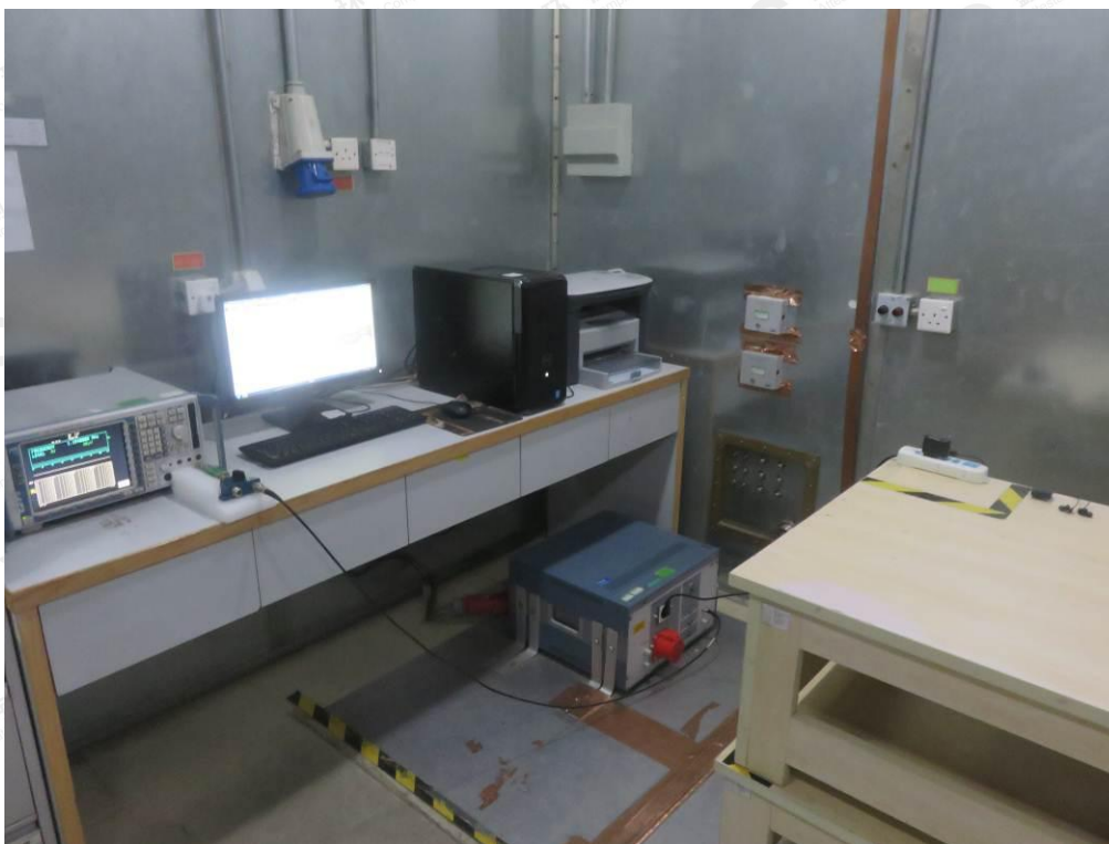
FCC RADIATED EMISSION TEST SETUP
