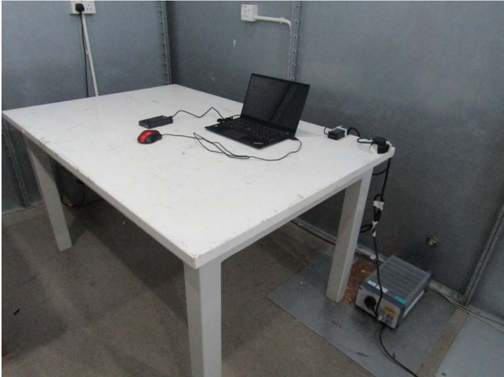
Measurement of Conducted Emission Test Set Up
