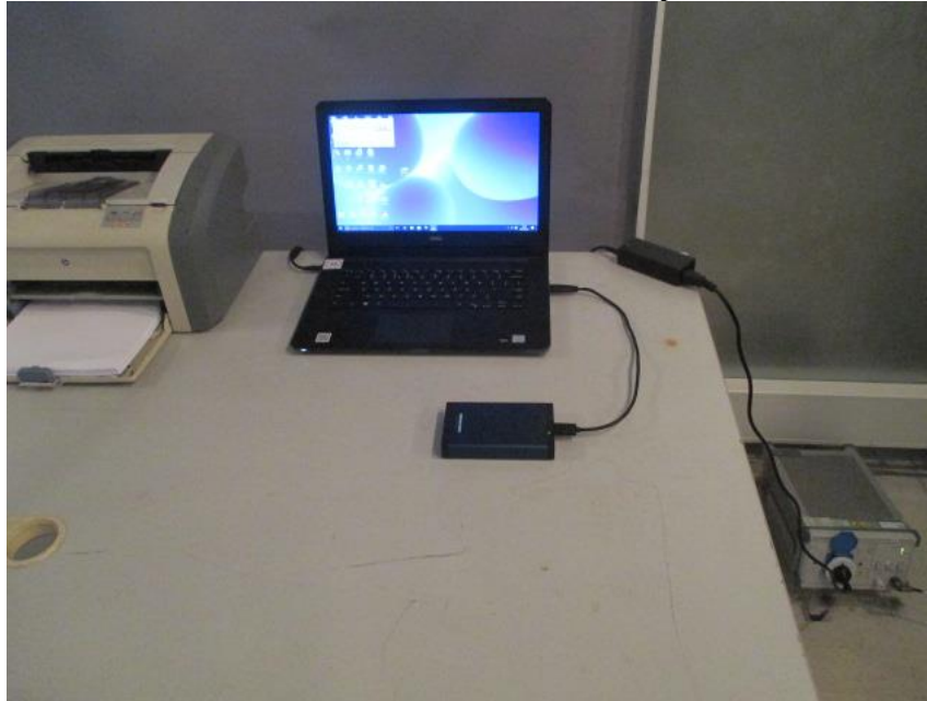
Conducted Emission Test Set Up
