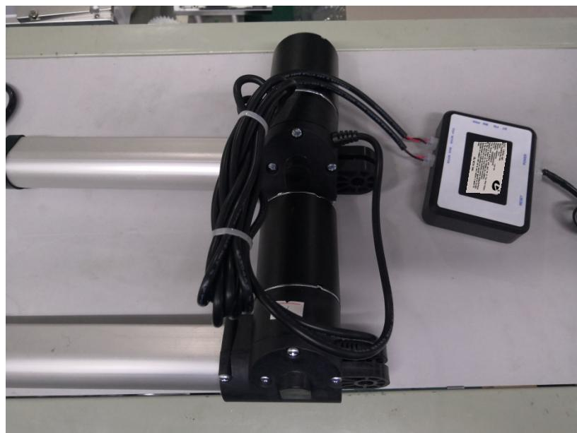
Then complete the mating pairing of the linear motor assembly and the control box assembly.
