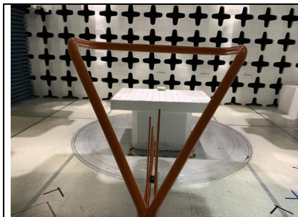
Radiated Emission Test below 1GHz Front View
