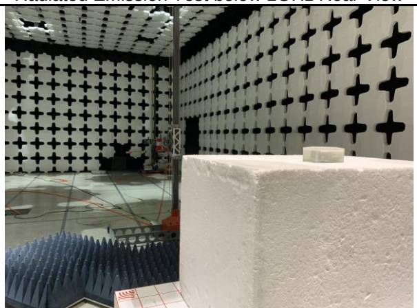
Radiated Emission Test above 1GHz Rear View
