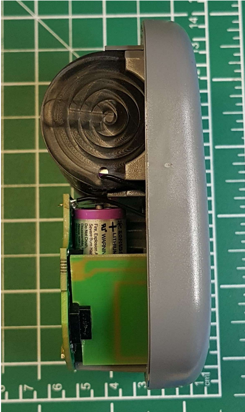
PCB with battery in enclosure side
