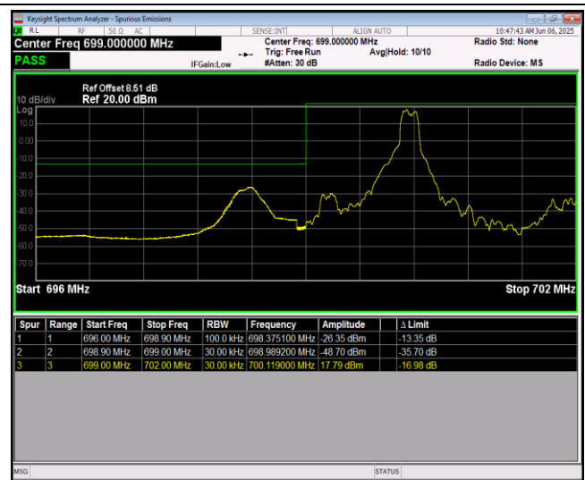
Band12-1.4MHz-QPSK-23173-1RB#0
