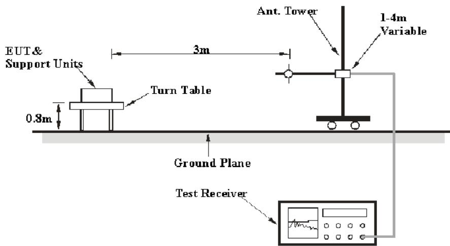
The radiated emission tests were performed in the 3-meter chamber a test site, using the setup accordance with the ANSI C63.10-2020. The specification used was the FCC Part 15.225, 15.209, 15.205, RSS-210 and RSS-Gen limits.
