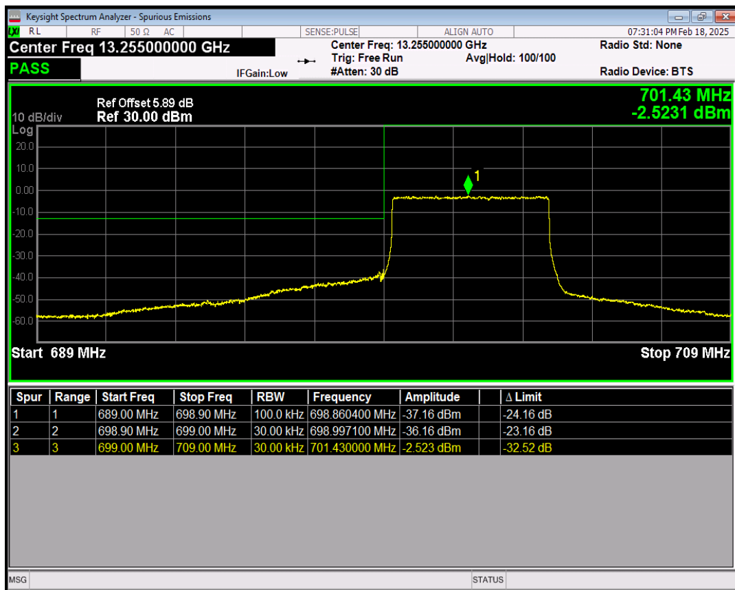
Band12 16QAM BW=5MHz Channel=23035 RB Size=1 Position=#0
