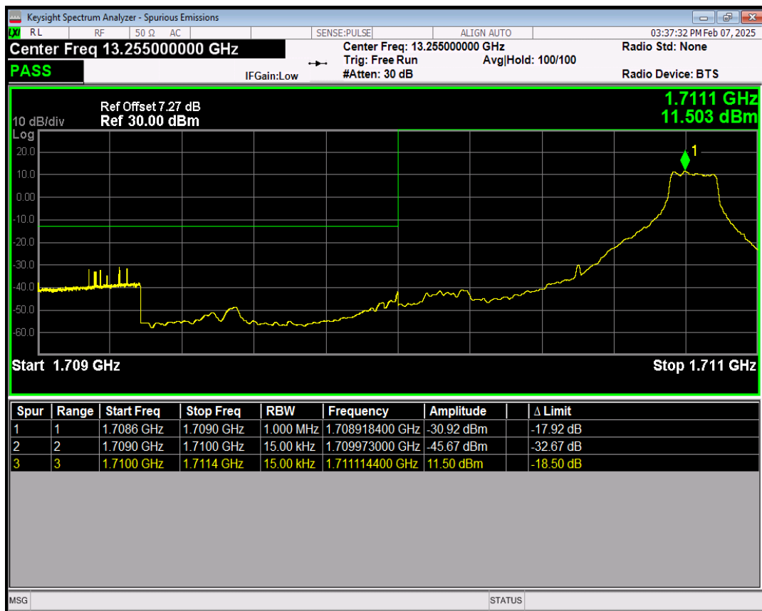
Band4 16QAM BW=1.4MHz Channel=19957 RB Size=6 Position=#0
