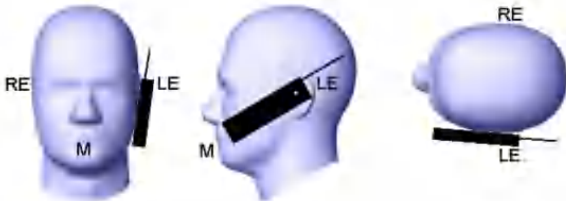
Fig 7.2.3 cheek or touch position. The reference points for the right ear (RE), left ear (LE), and mouth (M), which establish the Reference Plane for handset positioning, are indicated.
