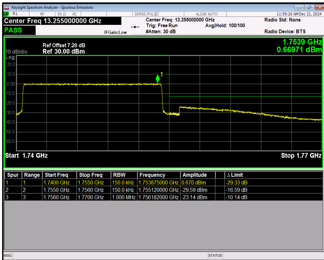
Band4 QPSK BW=20MHz Channel=20050 RB Size=1 Position=#0
