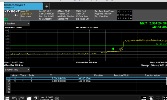
Out Of Band Emission IEEE 802.11ax_Channel 3_40MHz_Antenna 0_RU&Index SU
