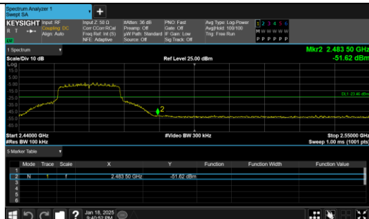
Out Of Band Emission IEEE 802.11ax_Channel 11_20MHz_Antenna 0_RU&Index SU
