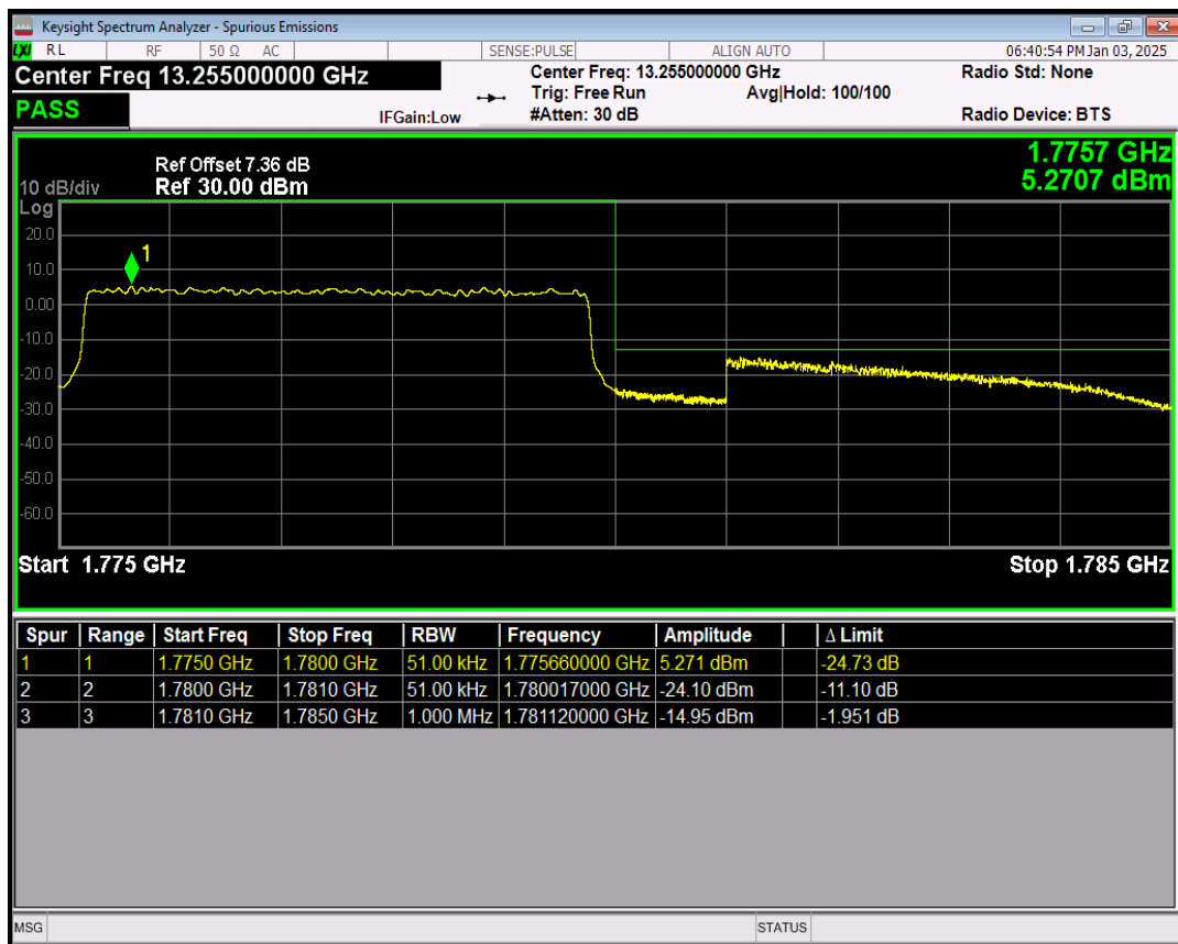
Band66 16QAM BW=5MHz Channel=132647 RB Size=1 Position=#0
