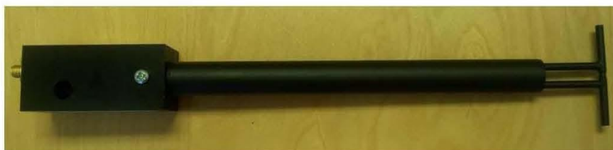
Figure 1 – MVG COMOSAR Validation Dipole
