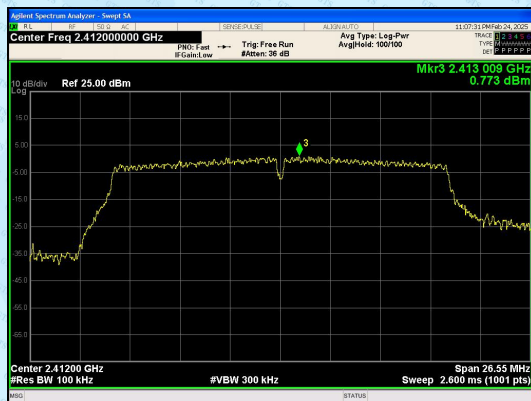
In-Band Reference Level IEEE 802.11n_Channel 1_20MHz_Antenna 0+Antenna 1
