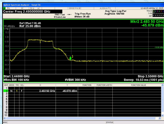
Out Of Band Emission IEEE 802.11n_Channel 11_20MHz_Antenna 0+Antenna 1
