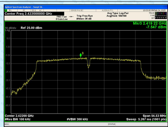
In-Band Reference Level IEEE 802.11n_Channel 3_40MHz_Antenna 0+Antenna 1
