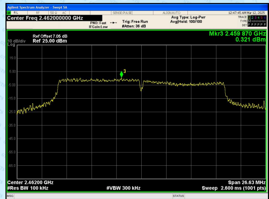
In-Band Reference Level IEEE 802.11n_Channel 11_20MHz_Antenna 0+Antenna 1
