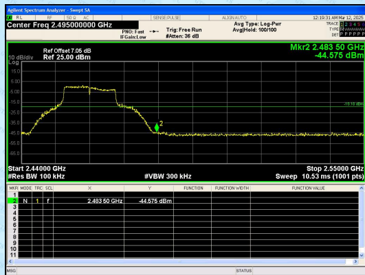
Out Of Band Emission IEEE 802.11g_Channel 11_20MHz_Antenna 0
