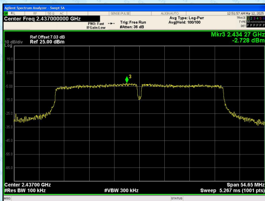
In-Band Reference Level IEEE 802.11n_Channel 6_40MHz_Antenna 0+Antenna 1
