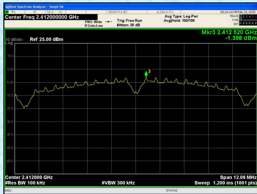
In-Band Reference Level IEEE 802.11b_Channel 1_20MHz_Antenna 0
