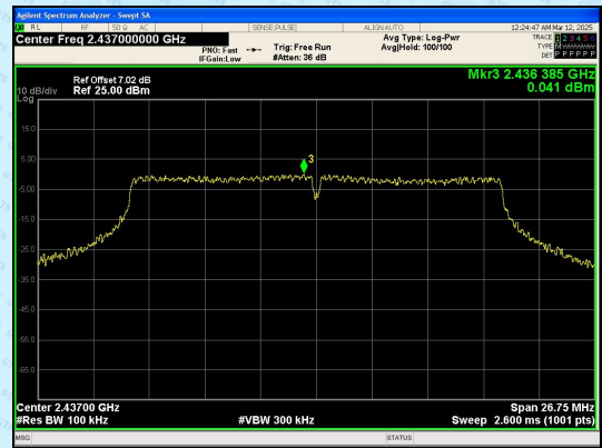
In-Band Reference Level IEEE 802.11n_Channel 6_20MHz_Antenna 0+Antenna 1
