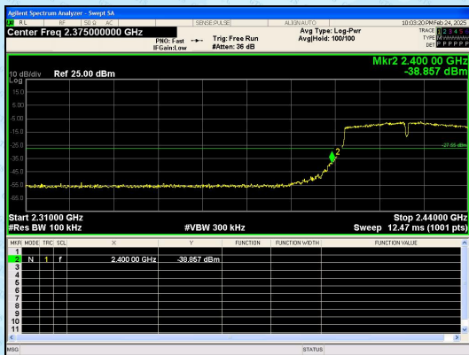
Out Of Band Emission IEEE 802.11n_Channel 3_40MHz_Antenna 0+Antenna 1
