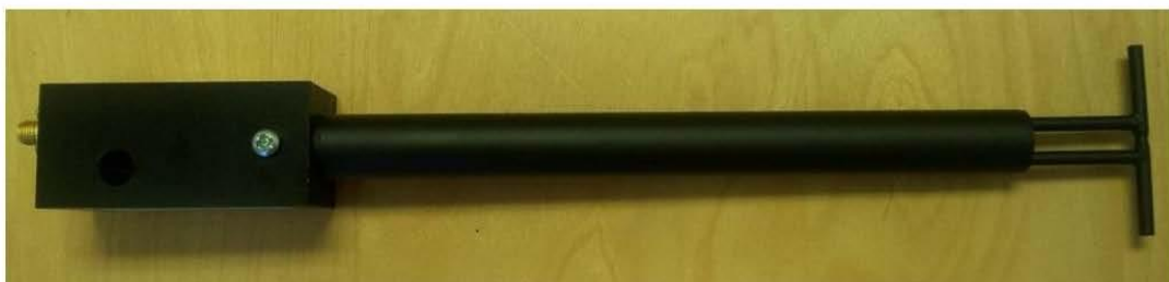
Figure 1 – MVG COMOSAR Validation Dipole
