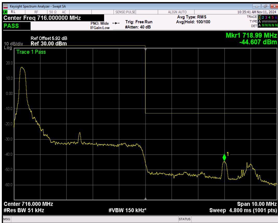
Band17 16QAM BW=5MHz Channel=23825 RB Size=1 Position=#Max
