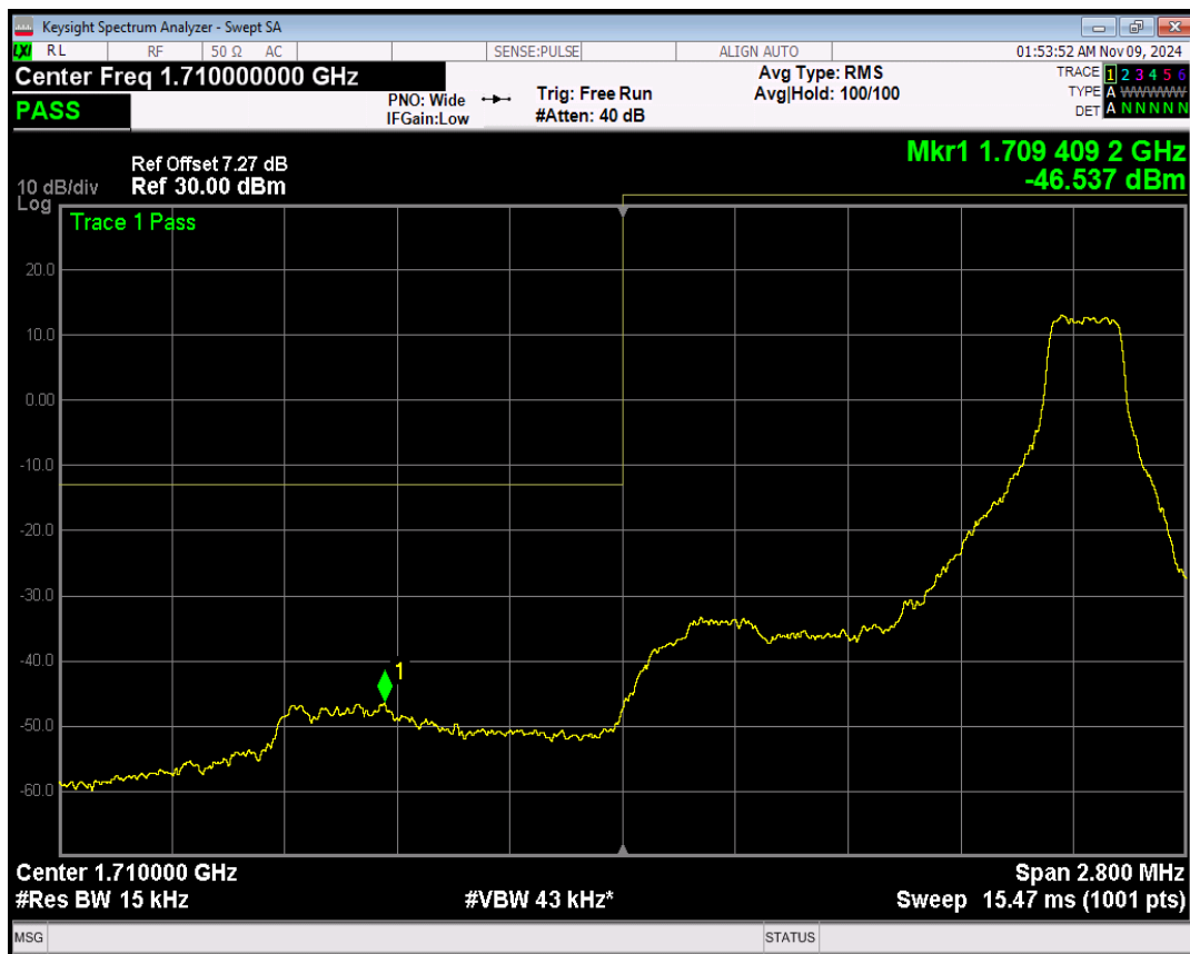
Band4 QPSK BW=1.4MHz Channel=19957 RB Size=6 Position=#0
