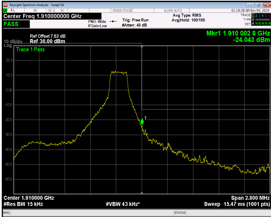
Band2 16QAM BW=1.4MHz Channel=19193 RB Size=6 Position=#0
