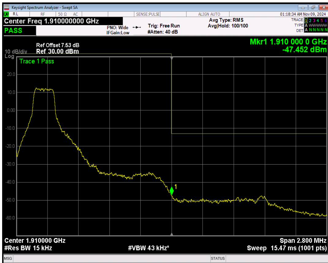
Band2 16QAM BW=1.4MHz Channel=19193 RB Size=1 Position=#Max
