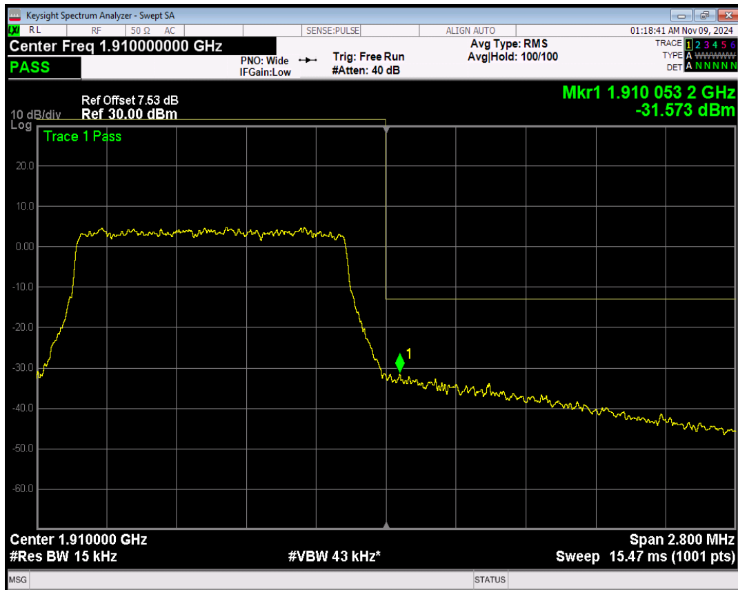
Band2 QPSK BW=3MHz Channel=18615 RB Size=1 Position=#0
