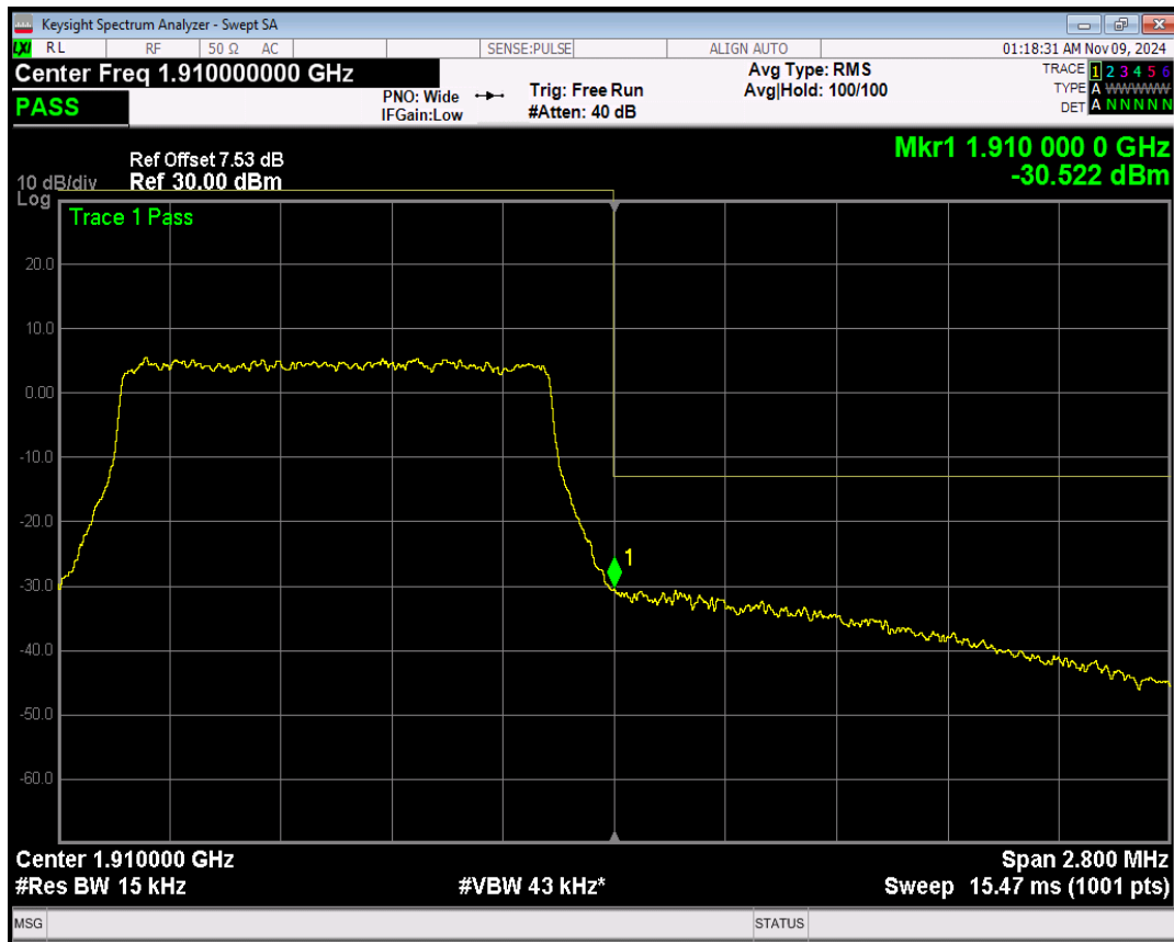
Band2 16QAM BW=1.4MHz Channel=19193 RB Size=1 Position=#0
