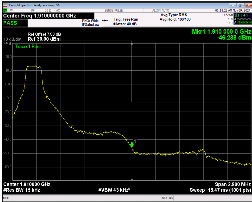
Band2 QPSK BW=1.4MHz Channel=19193 RB Size=1 Position=#Max
