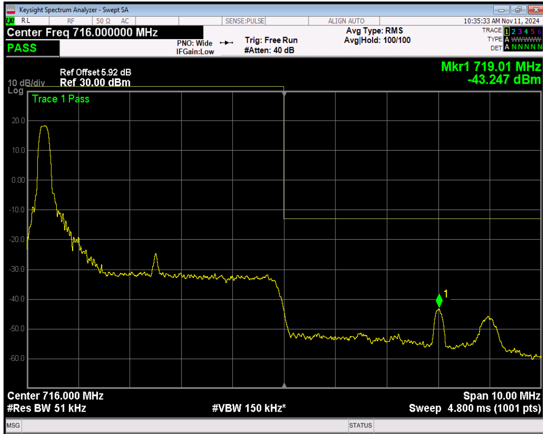
Band17 QPSK BW=5MHz Channel=23825 RB Size=1 Position=#Max
