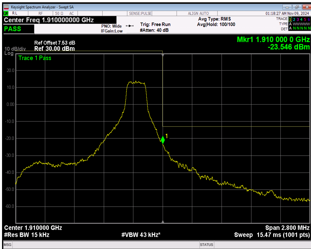
Band2 QPSK BW=1.4MHz Channel=19193 RB Size=6 Position=#0
