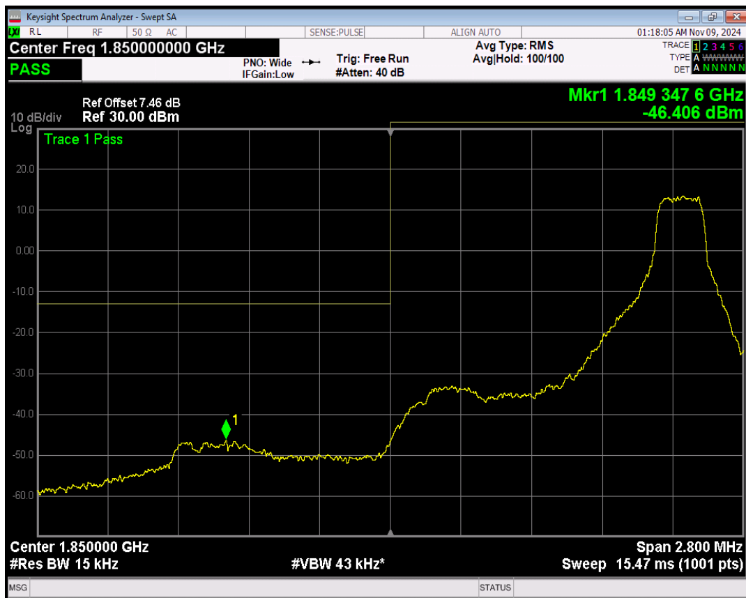
Band2 QPSK BW=1.4MHz Channel=18607 RB Size=6 Position=#0
