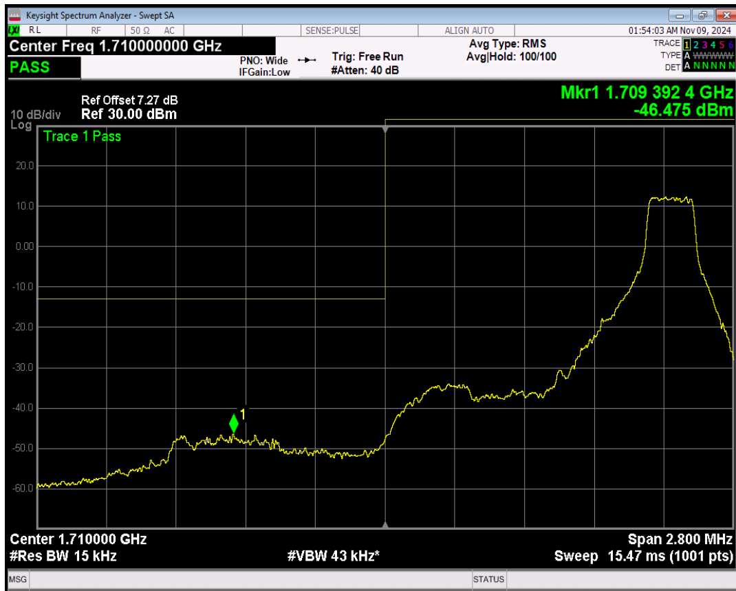
Band4 16QAM BW=1.4MHz Channel=19957 RB Size=6 Position=#0
