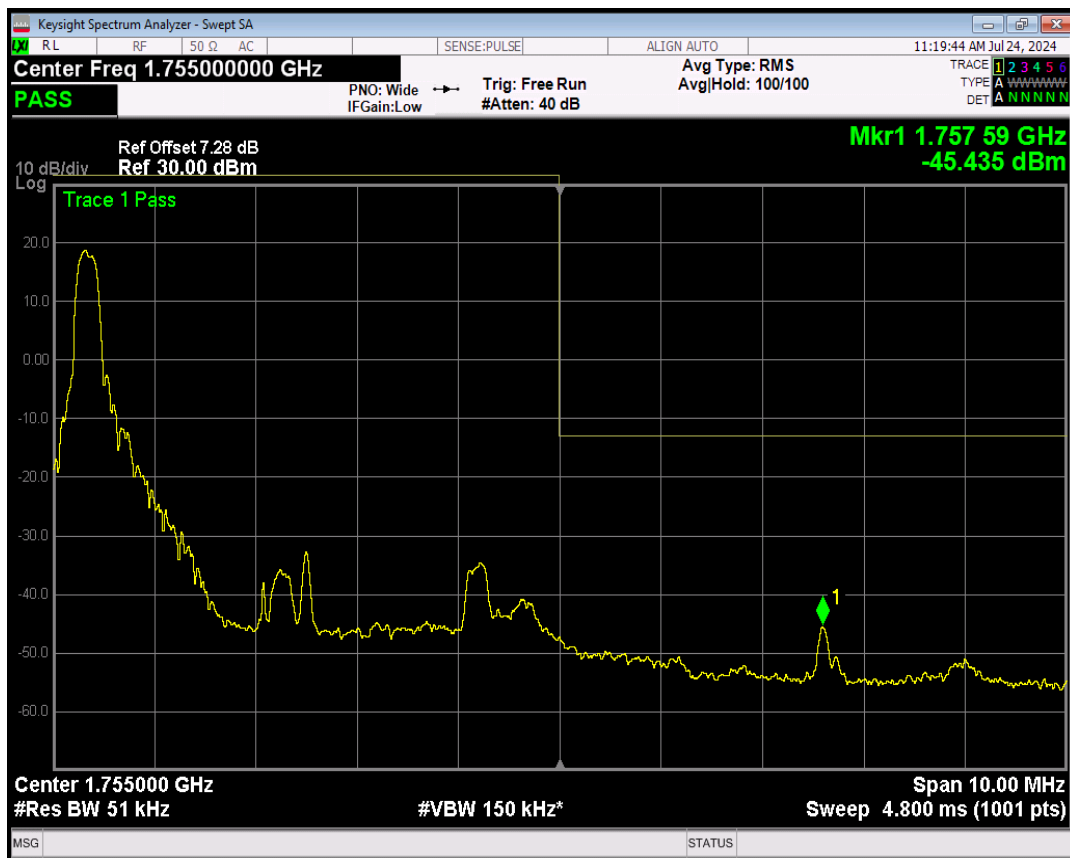
Band4 QPSK BW=5MHz Channel=20375 RB Size=1 Position=#Max
