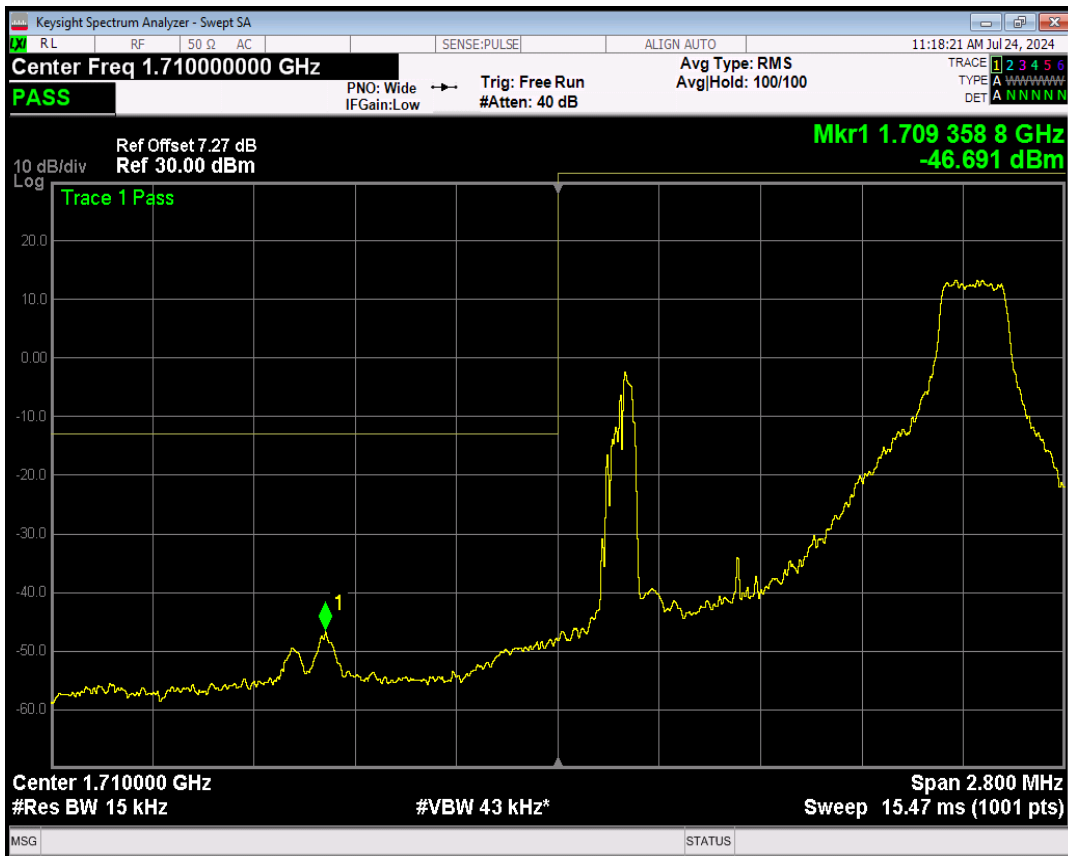
Band4 16QAM BW=1.4MHz Channel=19957 RB Size=6 Position=#0
