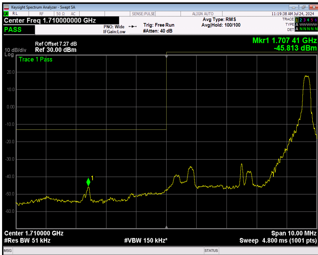
Band4 16QAM BW=5MHz Channel=19975 RB Size=25 Position=#0
