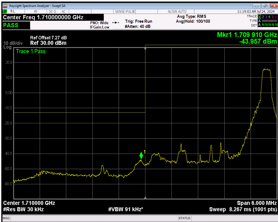
Band4 16QAM BW=3MHz Channel=19965 RB Size=15 Position=#0
