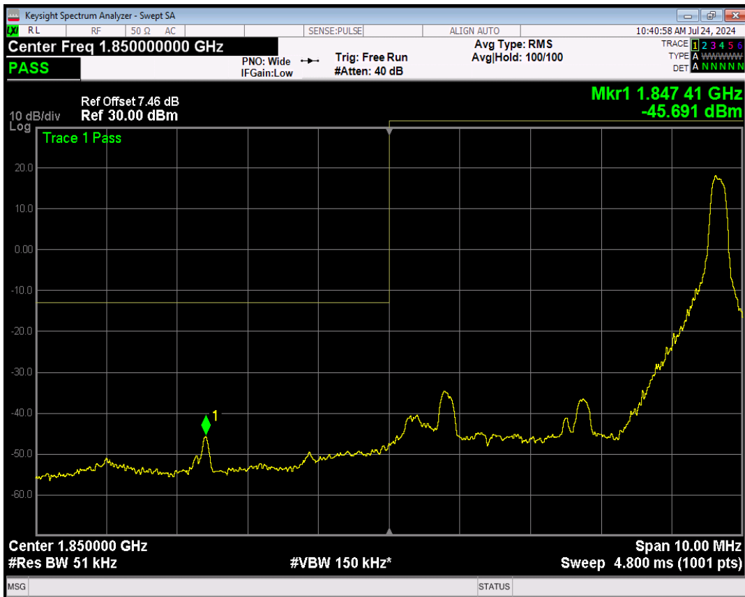
Band2 16QAM BW=5MHz Channel=18625 RB Size=25 Position=#0
