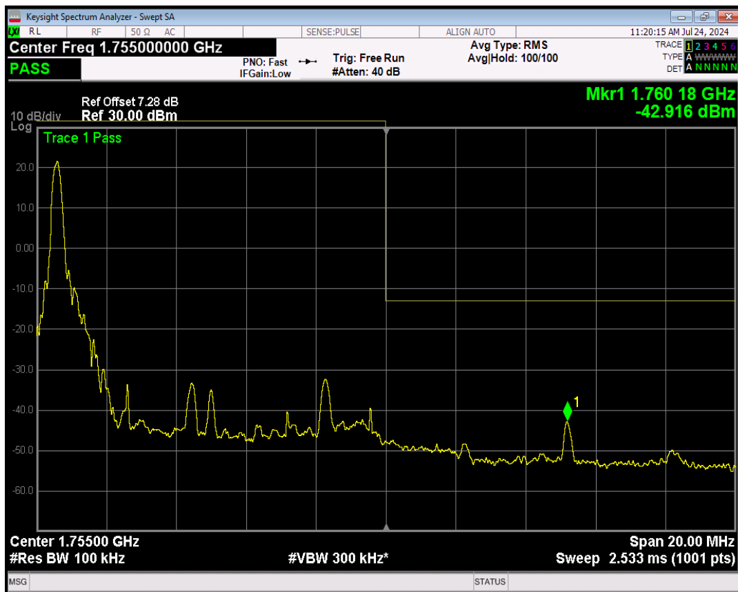
Band4 QPSK BW=10MHz Channel=20350 RB Size=1 Position=#Max
