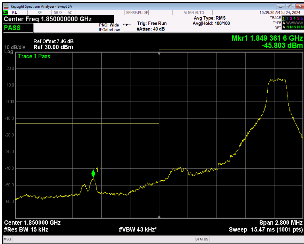
Band2 QPSK BW=1.4MHz Channel=18607 RB Size=6 Position=#0
