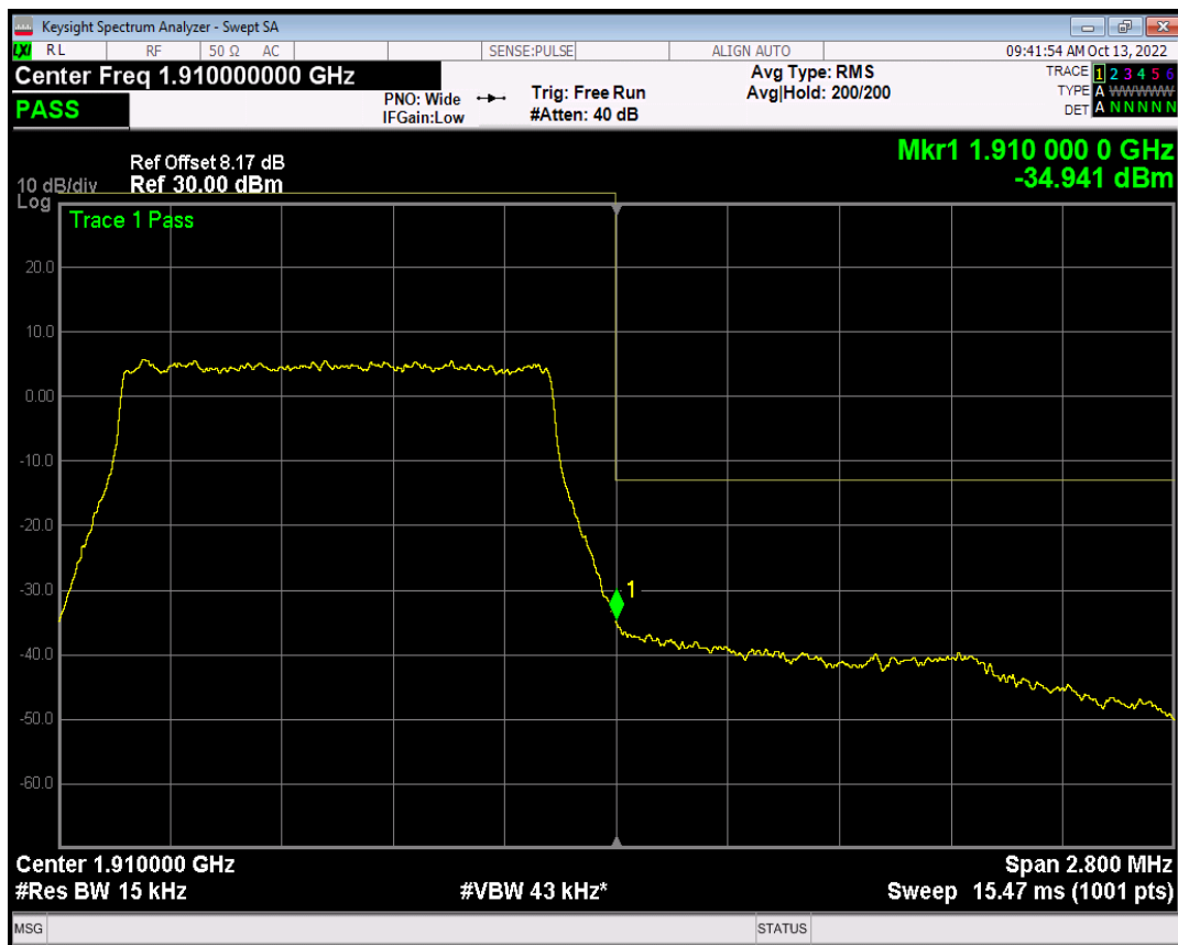
Band2 QAM16 BW=1.4MHz Channel=19193 RB Size=1 Position=#0
