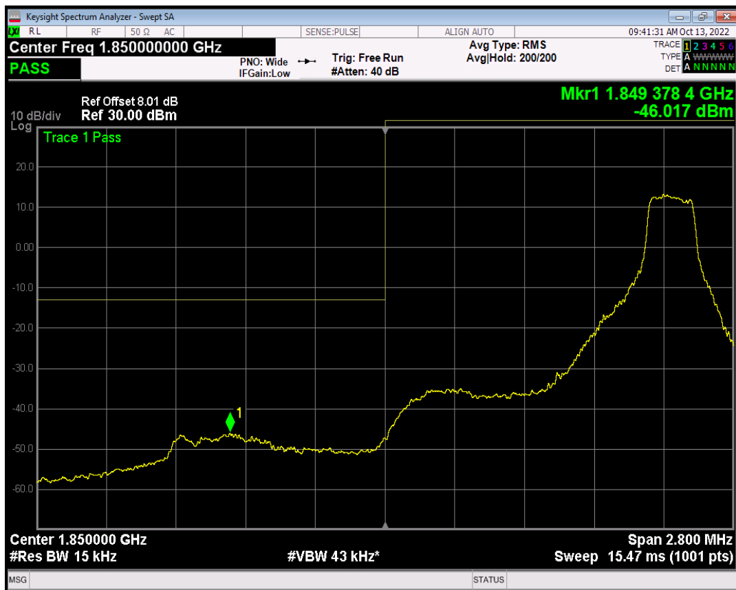
Band2 QAM16 BW=1.4MHz Channel=18607 RB Size=6 Position=#0
