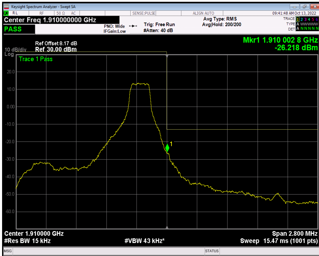
Band2 QPSK BW=1.4MHz Channel=19193 RB Size=6 Position=#0
