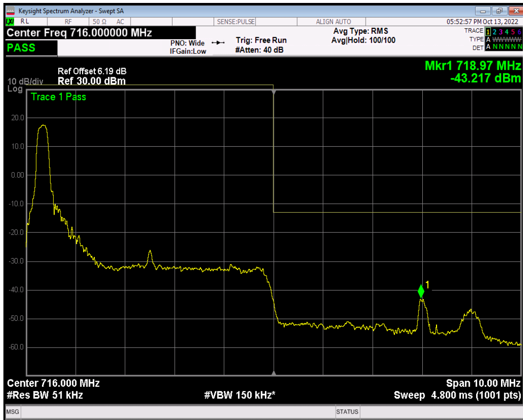
Band17 QAM16 BW=5MHz Channel=23825 RB Size=1 Position=#Max
