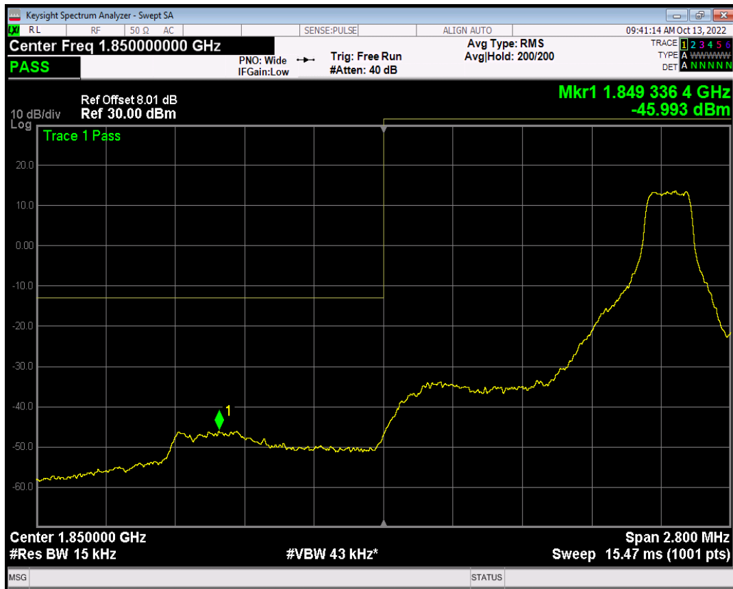
Band2 QPSK BW=1.4MHz Channel=18607 RB Size=6 Position=#0
