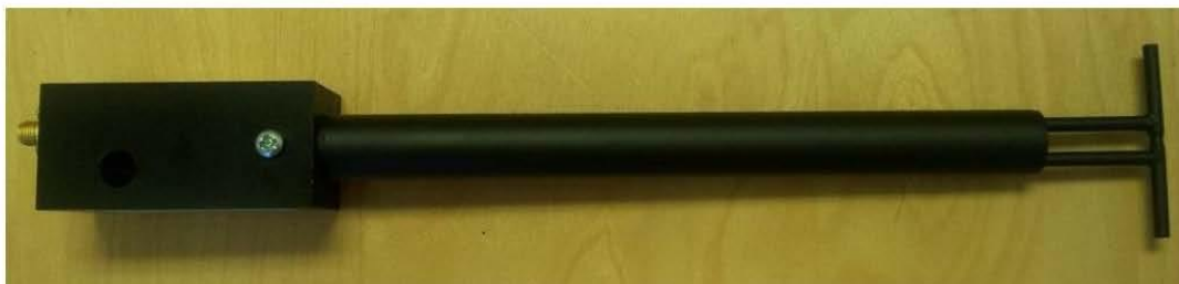
Figure 1 – MVG COMOSAR Validation Dipole
