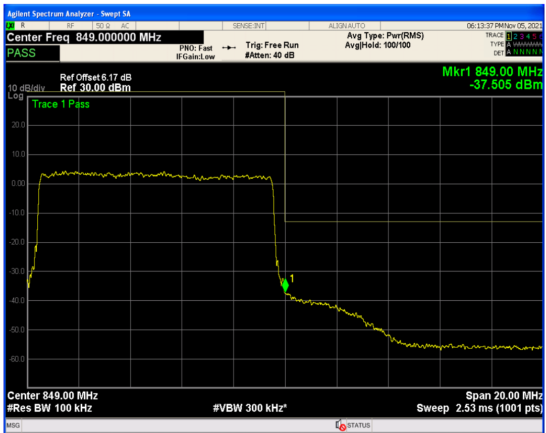
Band5 QPSK BW=10MHz Channel=20450 RB Size=50 Position=#0
