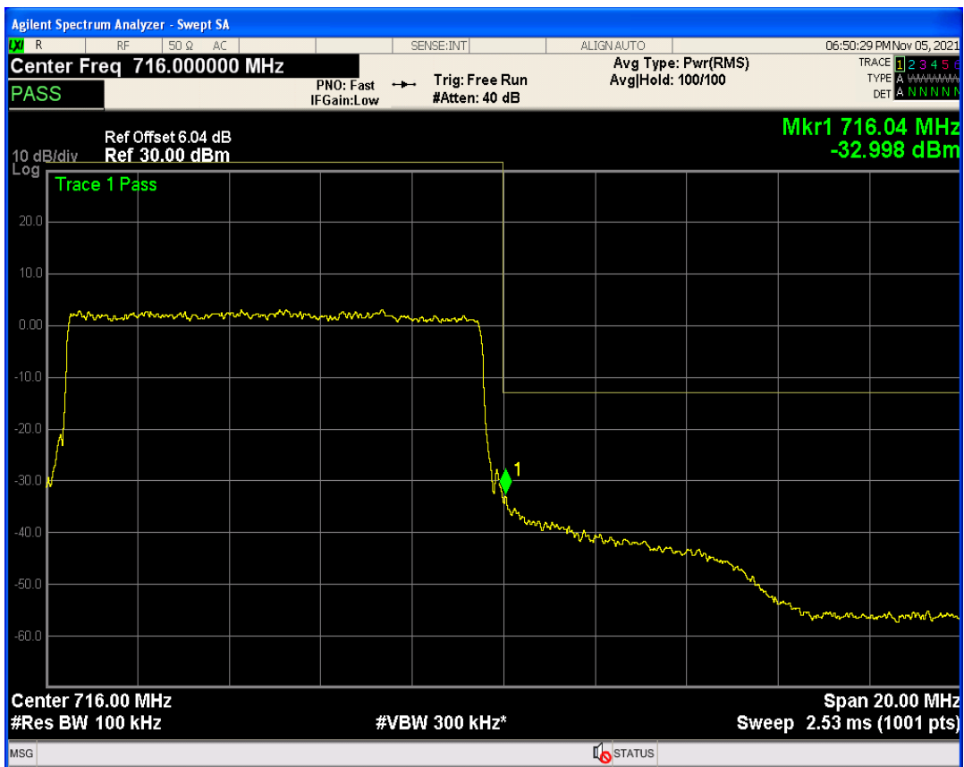
Band17 QAM16 BW=10MHz Channel=23800 RB Size=1 Position=#Max
