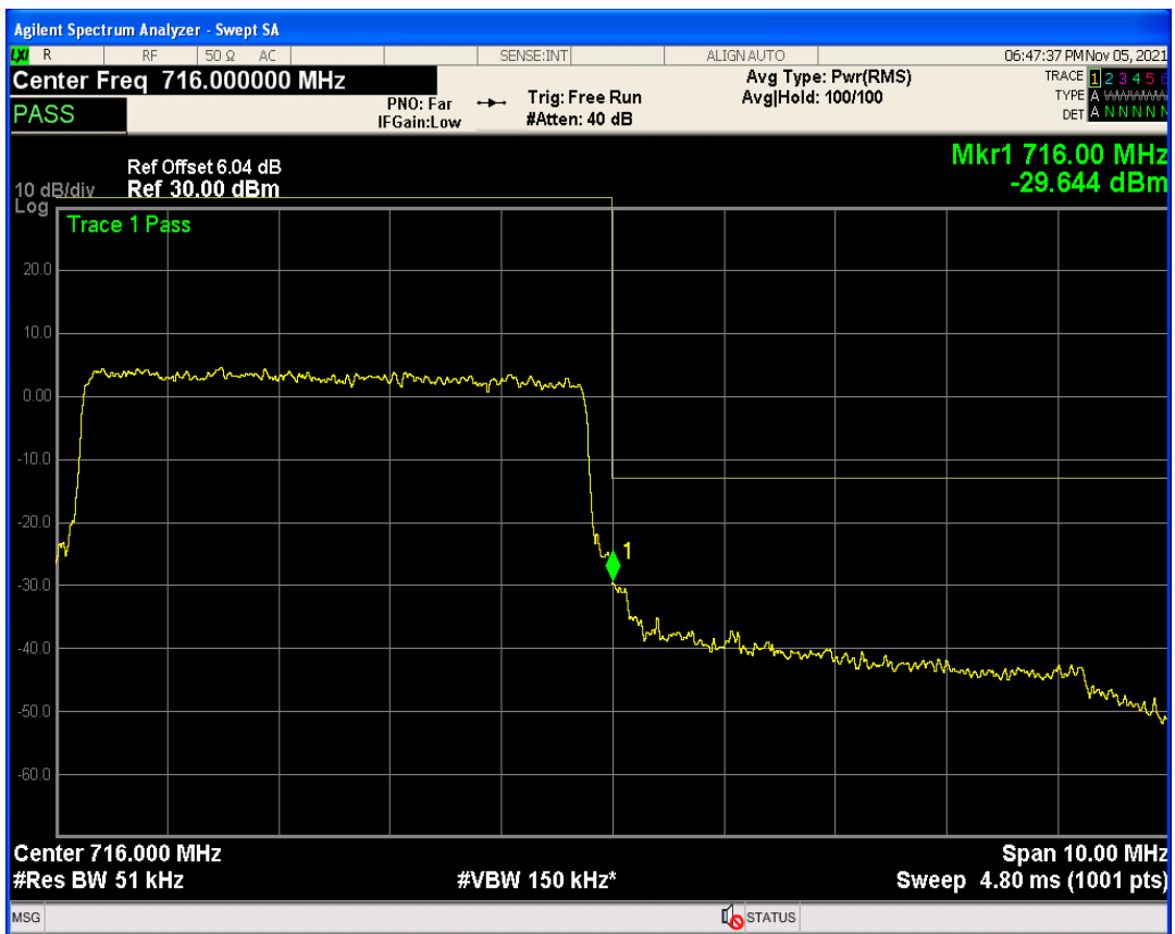
Band17 QPSK BW=5MHz Channel=23825 RB Size=1 Position=#Max
