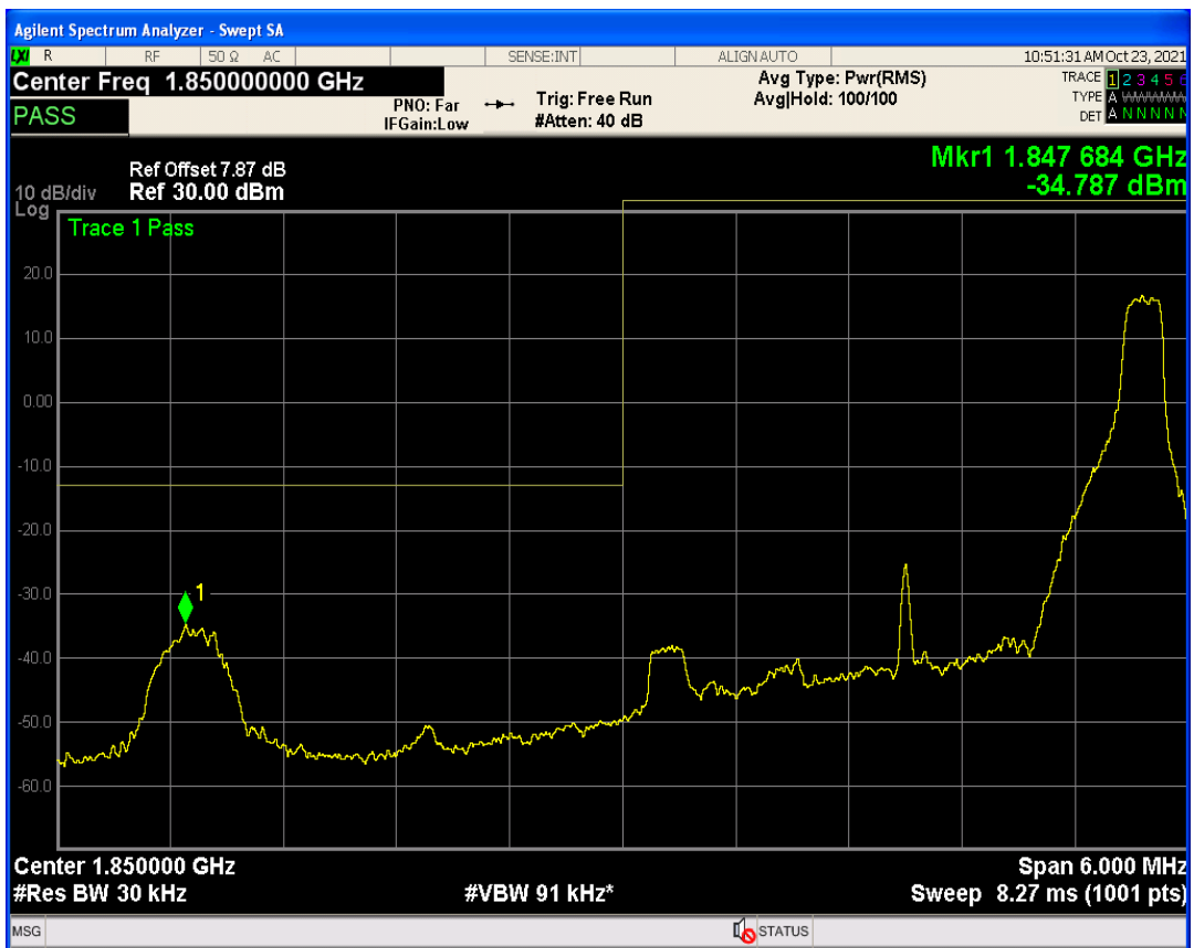
Band2 QPSK BW=3MHz Channel=19185 RB Size=1 Position=#Max
