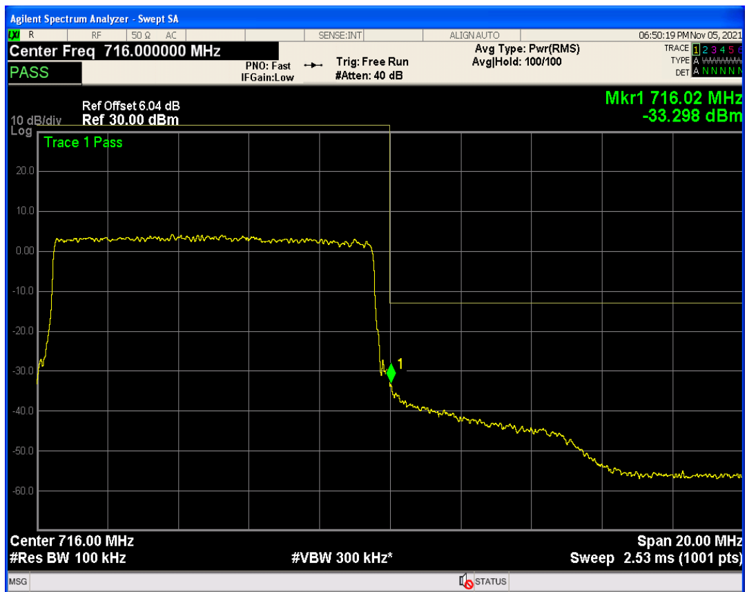
Band2 QPSK BW=1.4MHz Channel=18607 RB Size=1 Position=#0
