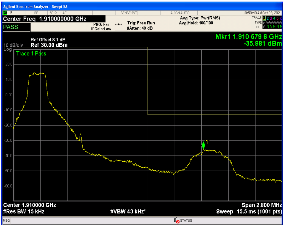
Band2 QPSK BW=1.4MHz Channel=19193 RB Size=1 Position=#Max
