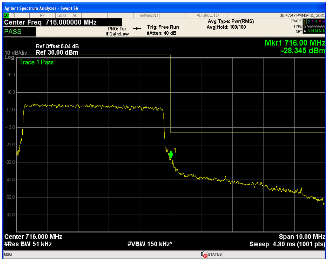
Band17 QPSK BW=10MHz Channel=23780 RB Size=50 Position=#0
