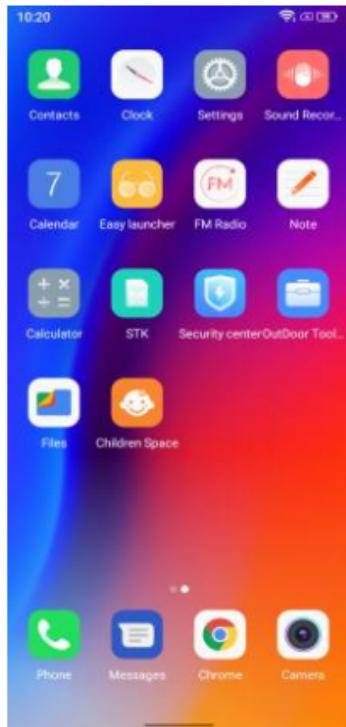
**2.3 Notification Bar:** At the top of the screen, the Status Bar displays the time, status, and notifications. If there is a new message, missed call or something in the notification bar, you can drag it down to open notification panel and click the desired one to have a view. When you finished, you can close it by dragging the panel up or pressing "Back".
