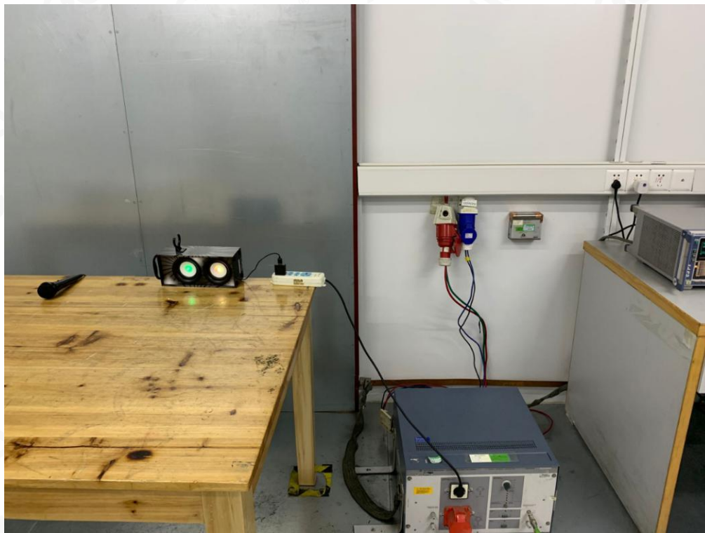
RADIATED EMISSION TEST SETUP BELOW 1GHZ
