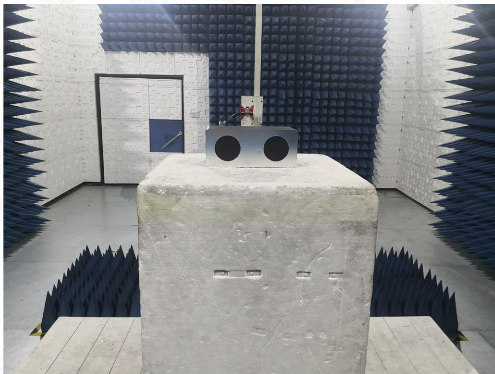
RADIATED EMISSION TEST SETUP ABOVE 1GHZ
