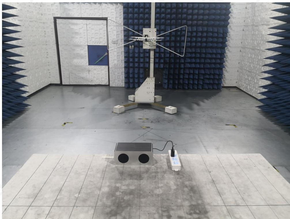
RADIATED EMISSION TEST SETUP ABOVE 1GHZ
