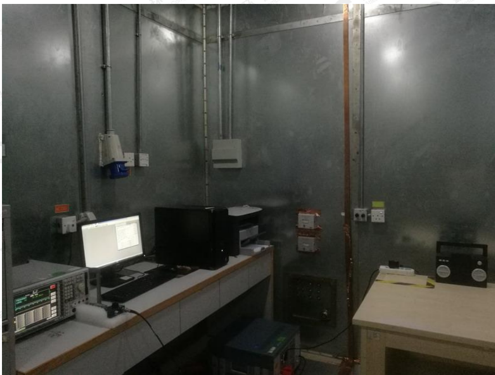
FCC RADIATED EMISSION TEST SETUP
