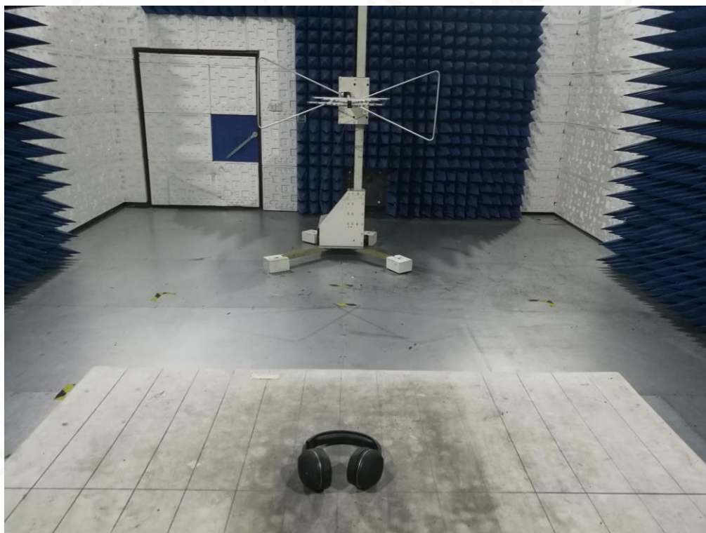
RADIATED EMISSION TEST SETUP ABOVE 1GHZ
