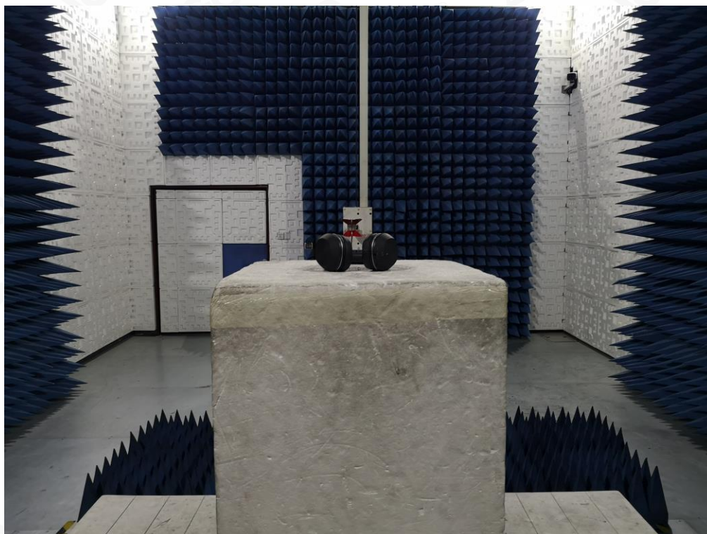
RADIATED EMISSION TEST SETUP ABOVE 1GHZ
