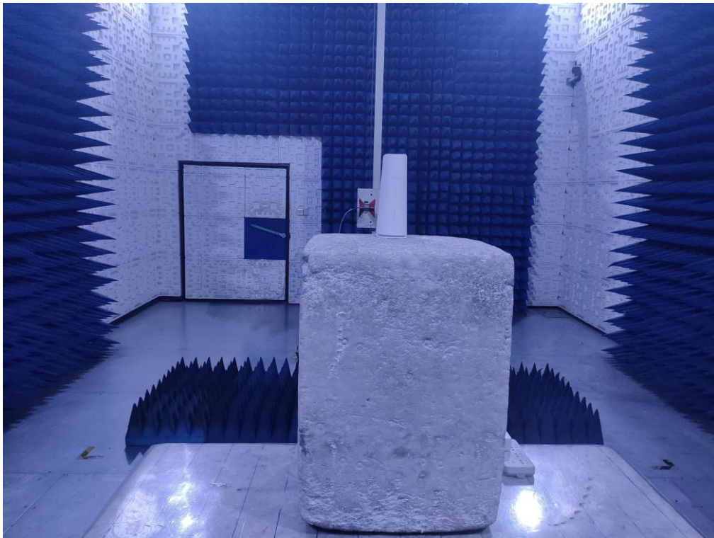
RADIATED EMISSION TEST SETUP ABOVE 1GHz
