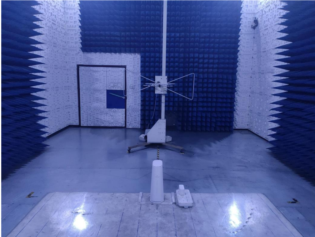
RADIATED EMISSION TEST SETUP ABOVE 1GHz
